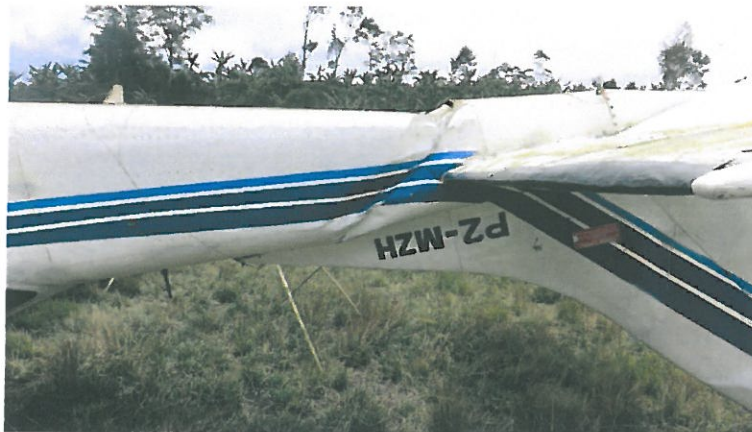
Figure 4: Damage to the tail section
