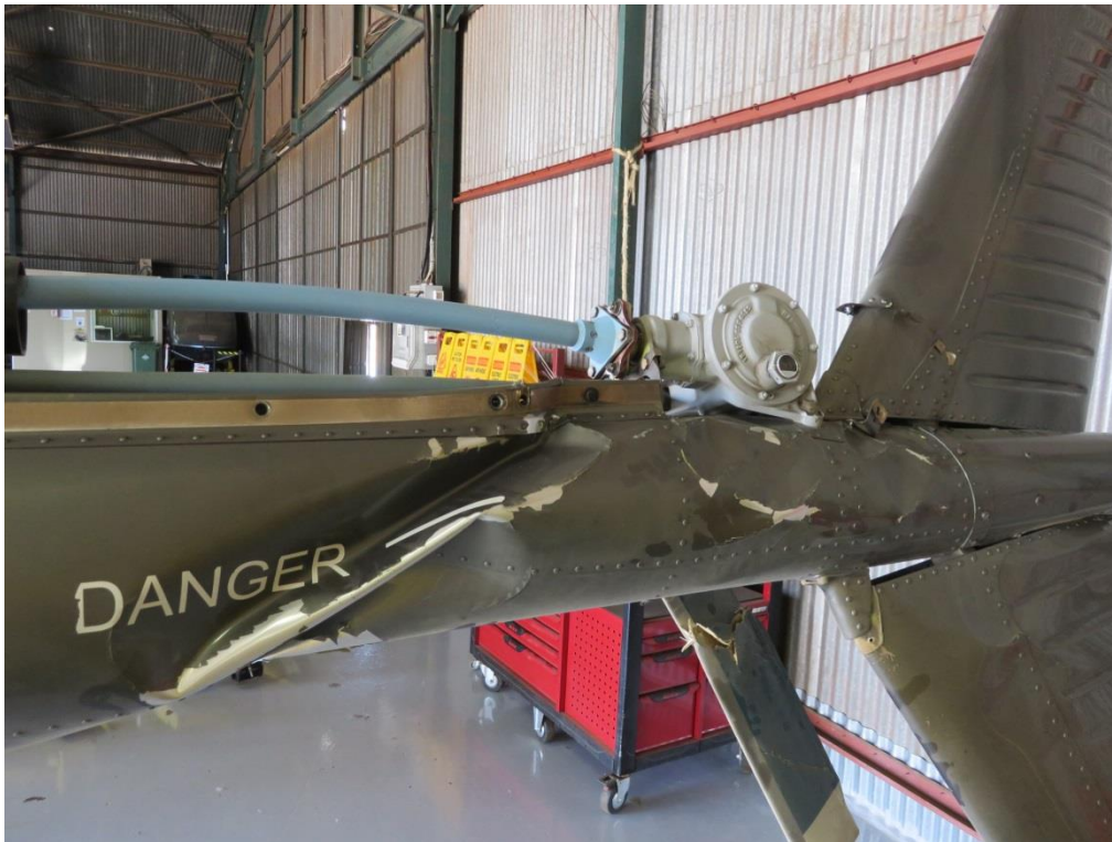
Figure 3: The twist to the aft tail boom structure
