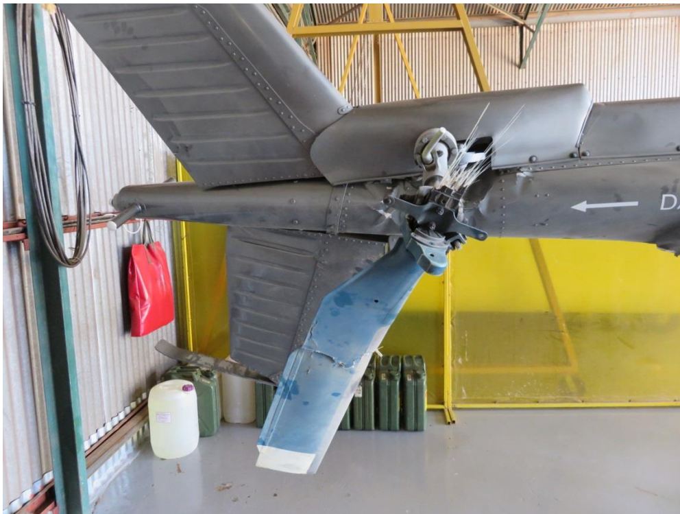
Figure 2: The damage to the tail rotor, with one of the blades broken off
