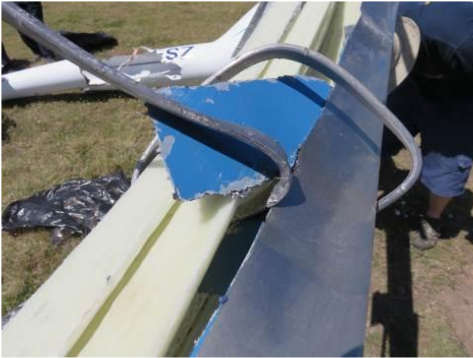
Figure 5. Deformation of leading edge lead balance weights of one of the main rotor blades
