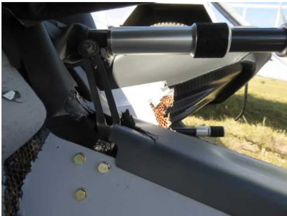
Figure 9. The collective pitch lever in the full up position
