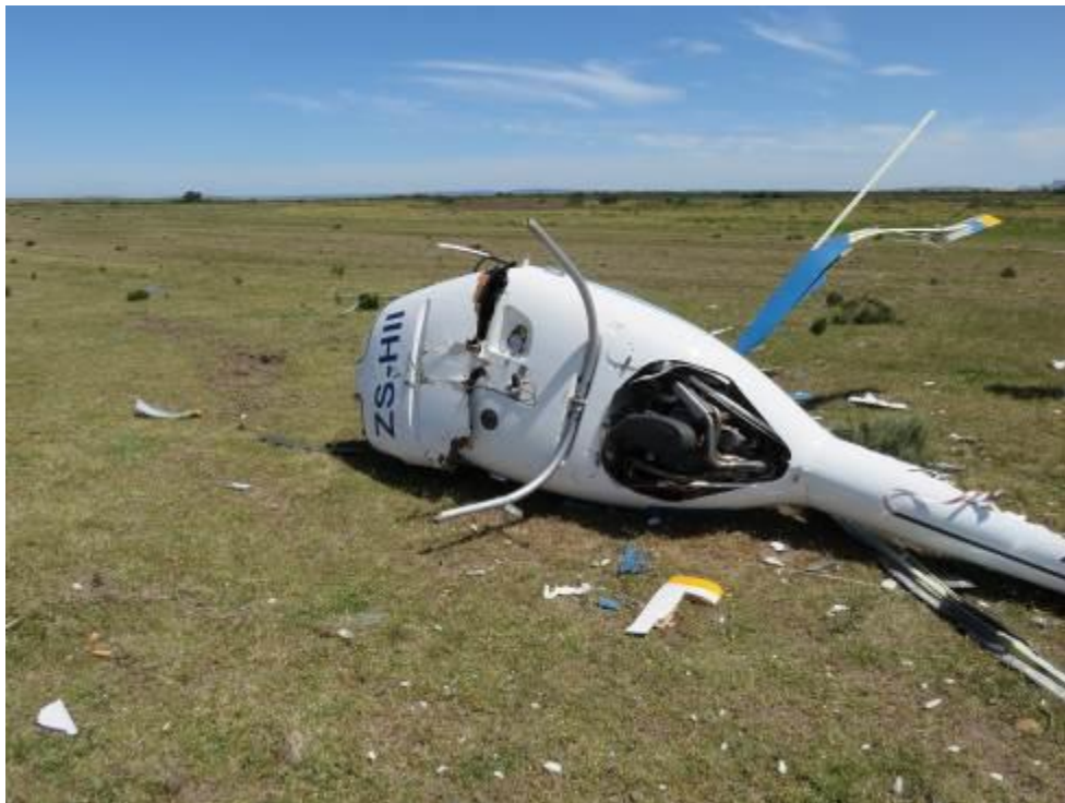
Figure 4. Lower fuselage, indicating the missing forward cross-tube and skid gear assembly
