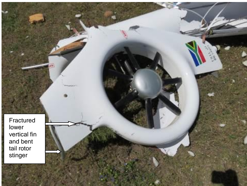
Figure 6. The vertical fin assembly and the shrouded tail rotor lying next to the tail boom
