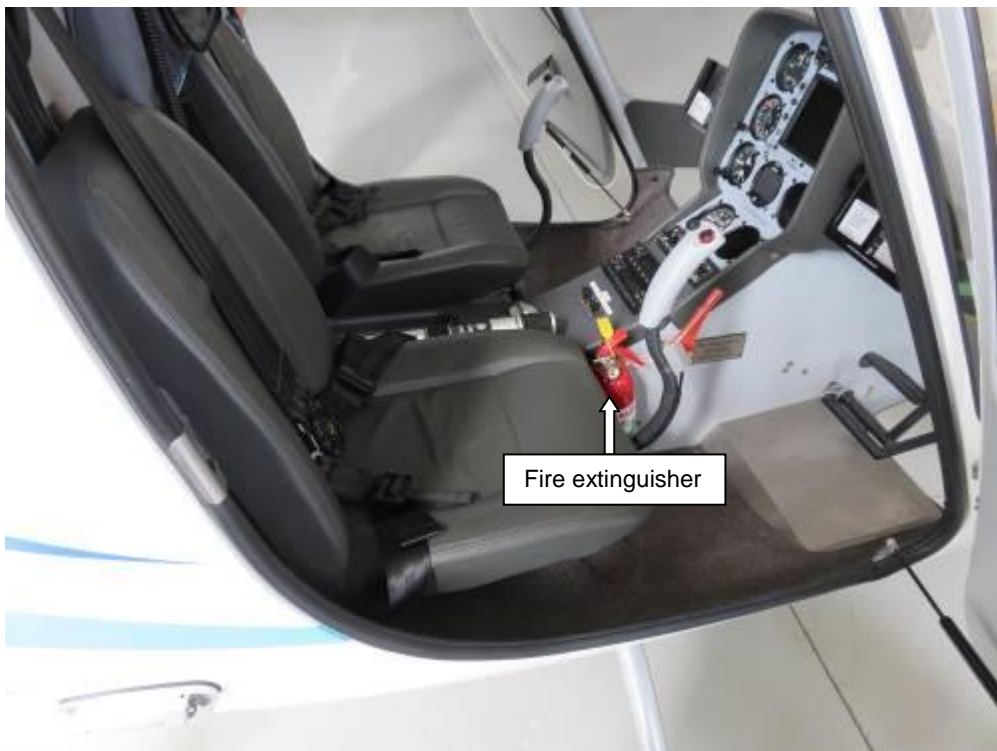
Figure 14. The portable in-cabin fire extinguisher (serviceable helicopter)
