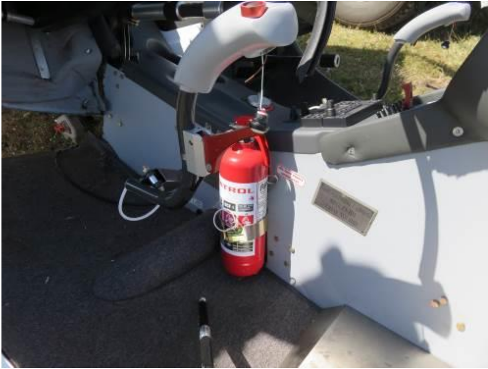
Figure 13. A view of the portable in-cabin fire extinguisher (accident helicopter)
