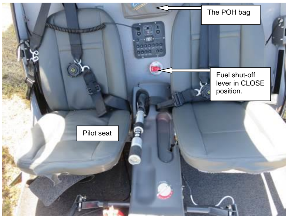
Figure 10. A view of the cockpit/cabin, where the seats absorbed the impact forces
