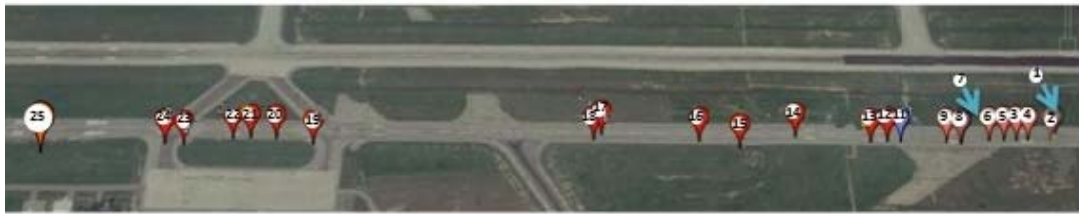
Aircraft ground track and location of dislodged parts
