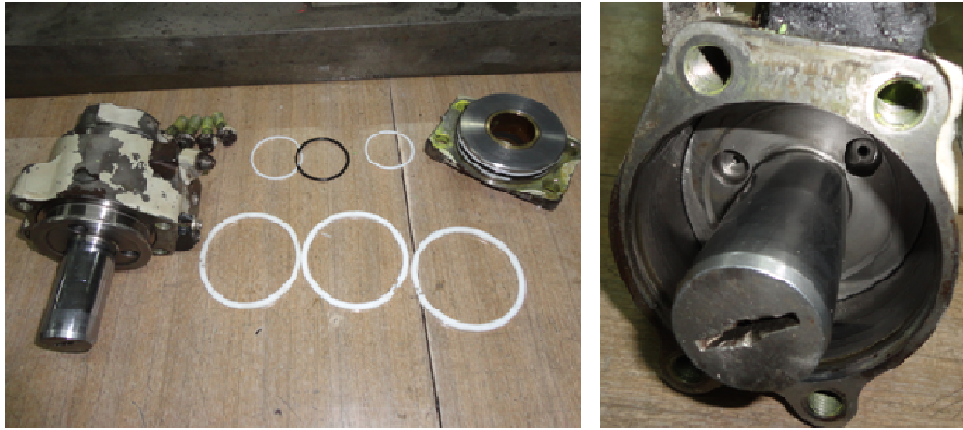
Shimmy damper internal seals and parts were found intact
