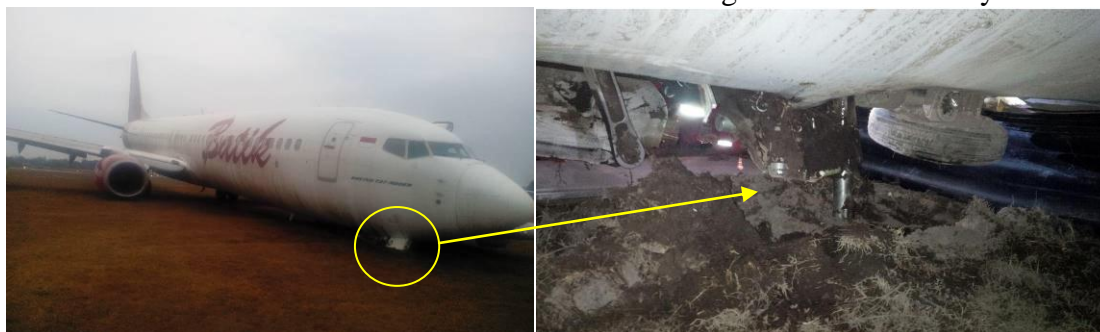
Figure 3: The aircraft after the impact with the nose wheel folded backward
