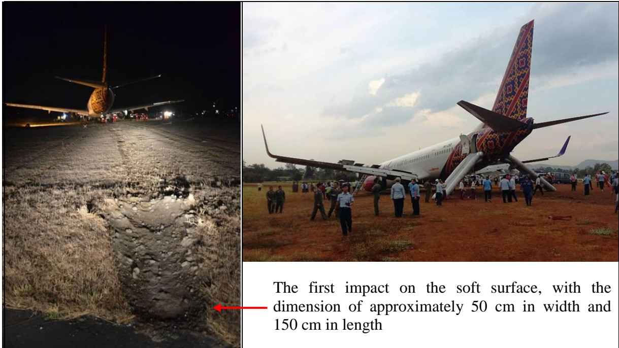
Figure 12: Nose wheel mark on the grass (left) and the Aircraft last position after passenger evacuated (right)
