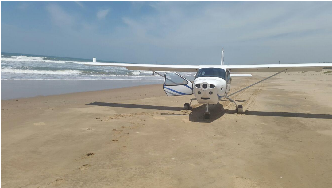
Figure 1: The aircraft as it came to a halt on the beach without a propeller
