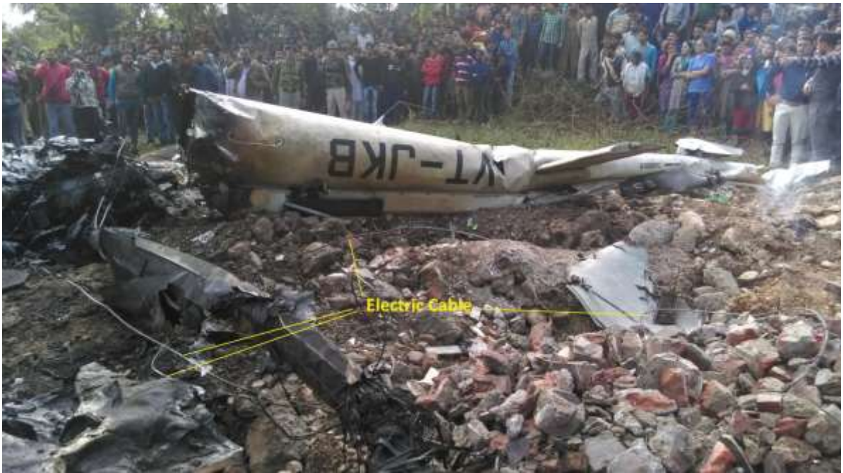
Broken electric cables were found under the wreckage and around it.
