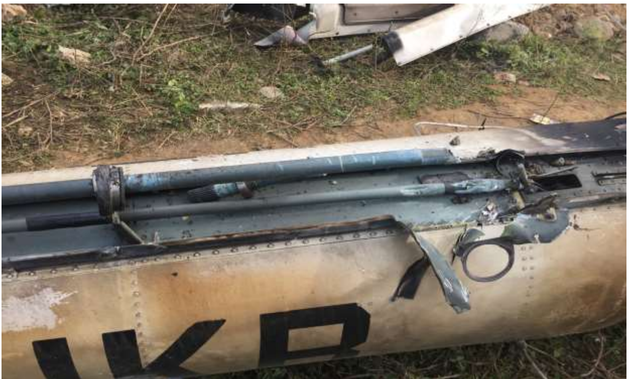
Tail rotor drive shaft was found broken
