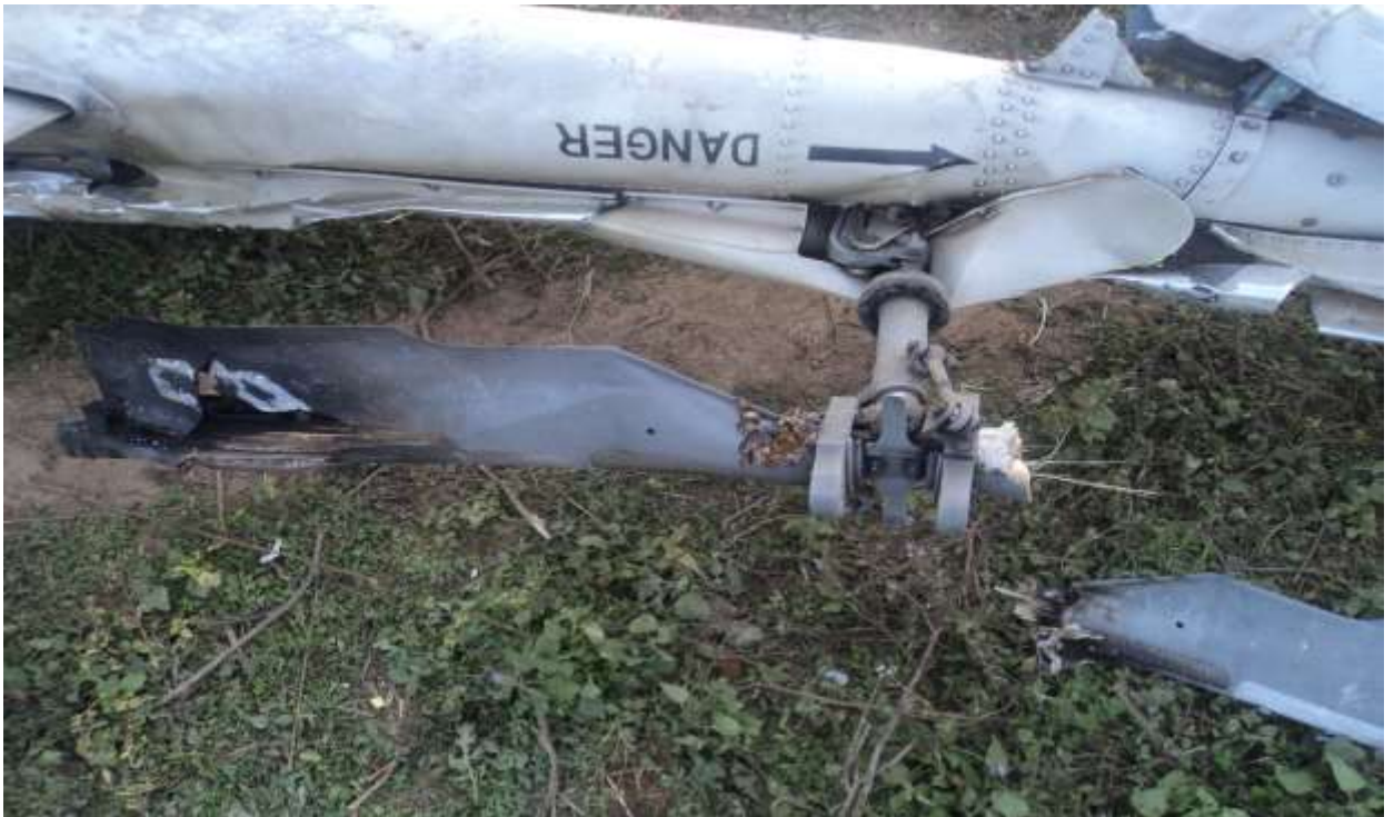
One of the tail rotor blades severed from the tail rotor hub
