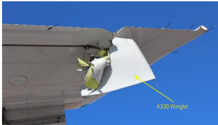
Figure 2. Right wingtip of the B777 with part of the embedded A330 winglet
