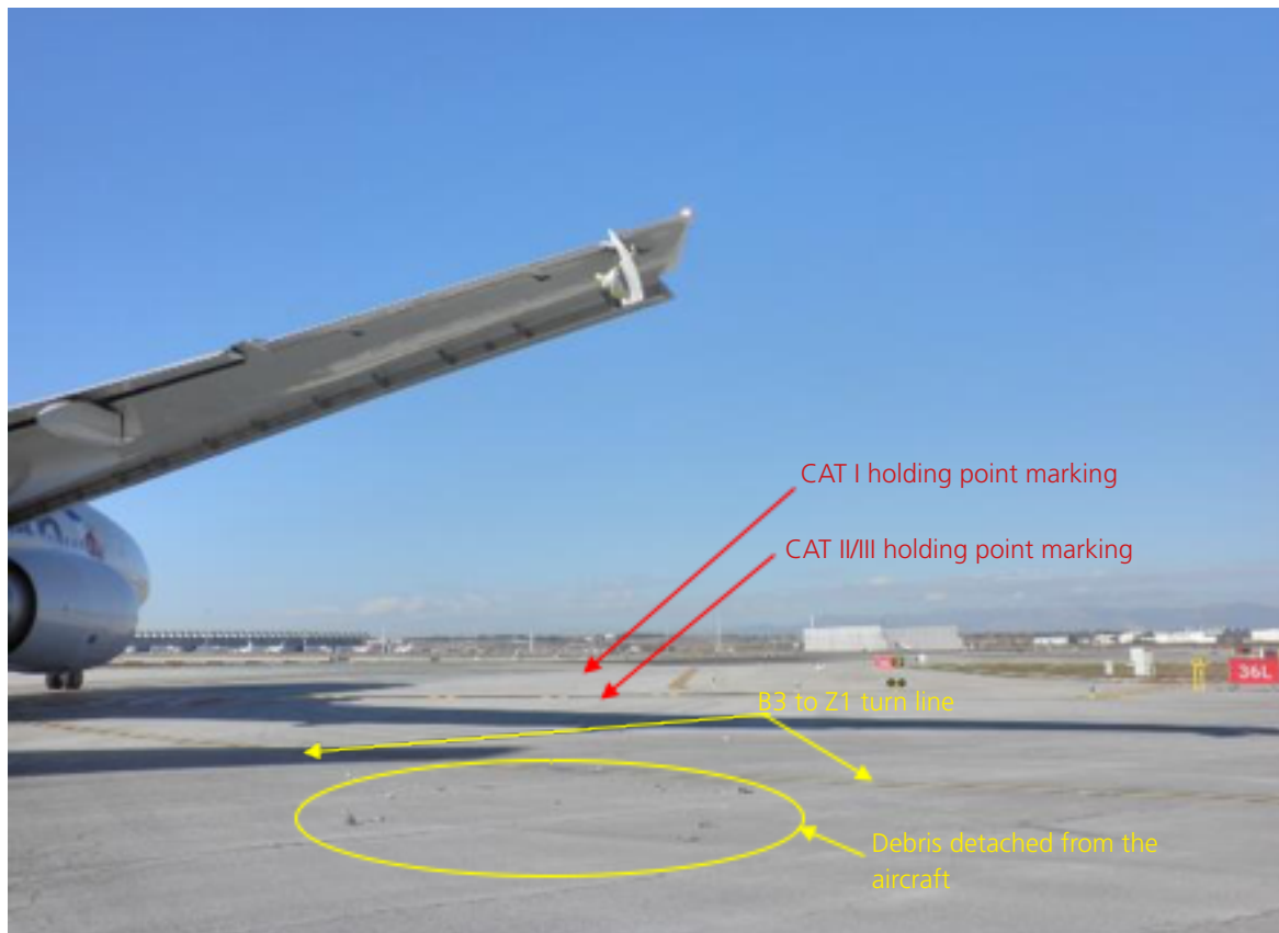
Figure 14. Photograph of aircraft N758AN on taxiway Z1, taken before it was moved and after being impacted by aircraft EC-LZX
