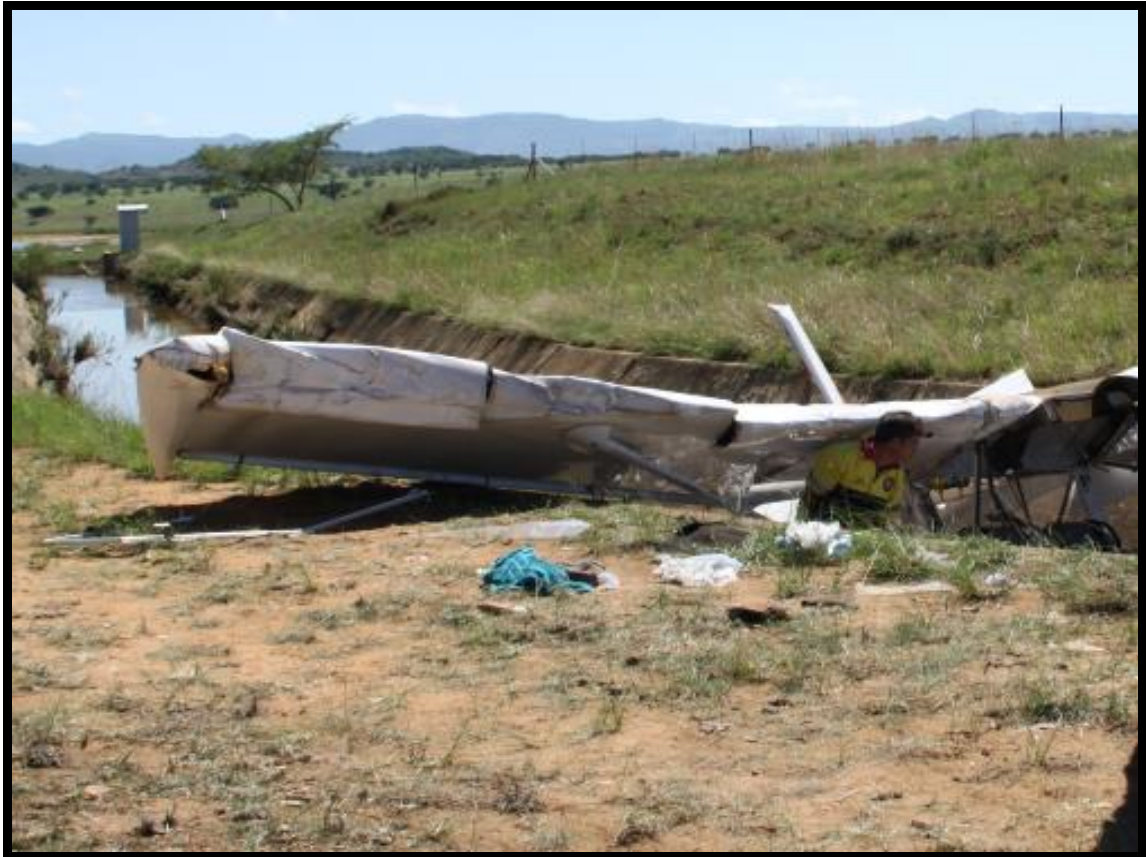
Figure 5: Shows damages on the right wing
