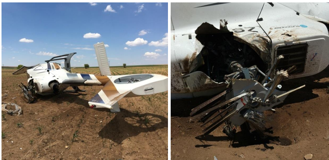
Figure 11: Photographs showing the final position of the rotor head
