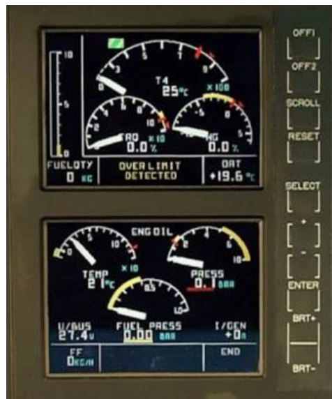
Figure 5: VEMD computer unit installed on the helicopter
