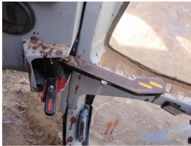
Figure 12: The position of the fuel shut-off lever
