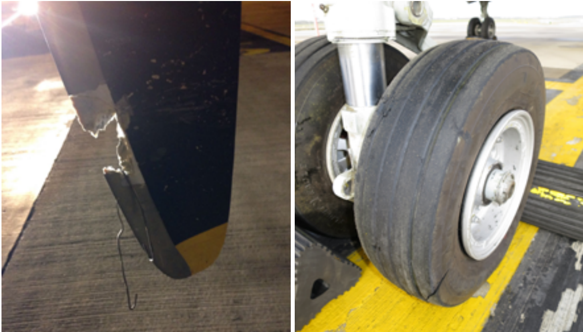
Figure 3: Right-hand engine propeller with wire embedded on arrival at Stansted airport (left image). Aeroplane nose wheel, as seen from the front side of the aeroplane, with port wheel damaged (right image). (Photo: AAIB)
