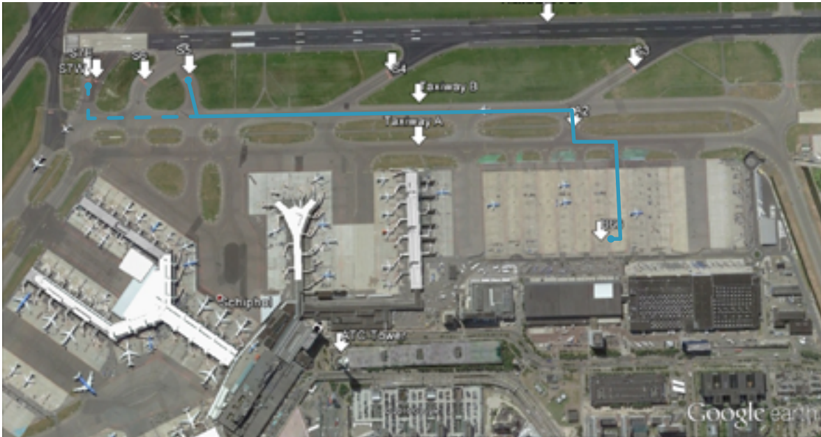
Figure 1: Overview of the relevant part of Amsterdam Airport Schiphol with the parking stand, taxiways and Runway 24 together with a rough representation of the intended (blue dashed) and actual taxiing track (blue). (Photo: Google Earth)
