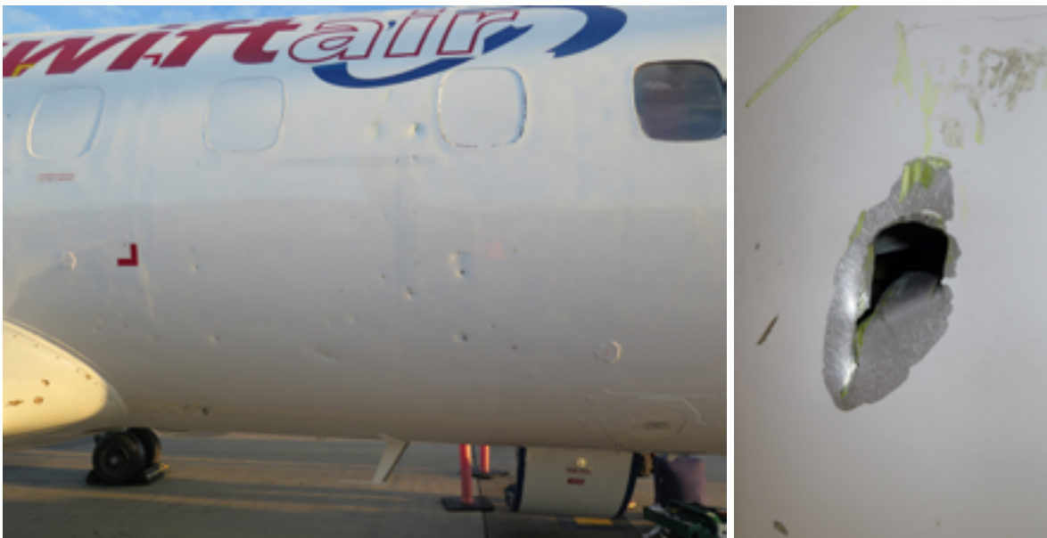
Figure 2: Fuselage on the right-hand side of the aeroplane with the hole pattern (left) and a detailed view of the punctured fuselage with visible yellow paint deposits (right). (Photo: AAIB)
