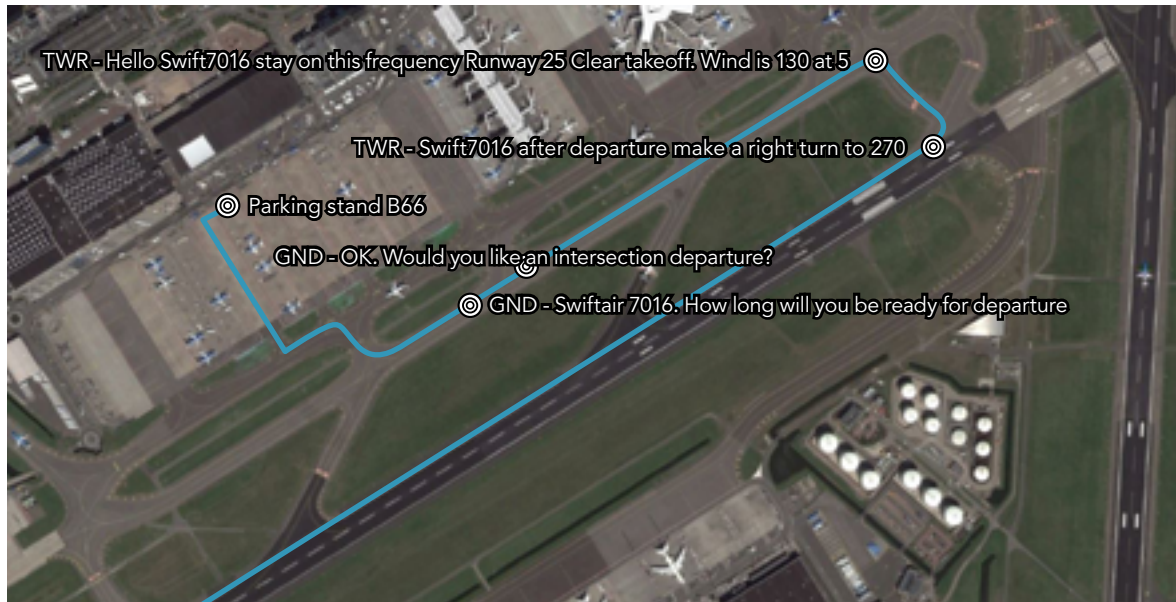
Figure 11: Actual taxi and take-off track of the aeroplane, reconstructed from radar data, together with a transcript of the relevant communication between ATC and the flight crew. (Photo: Google earth)
