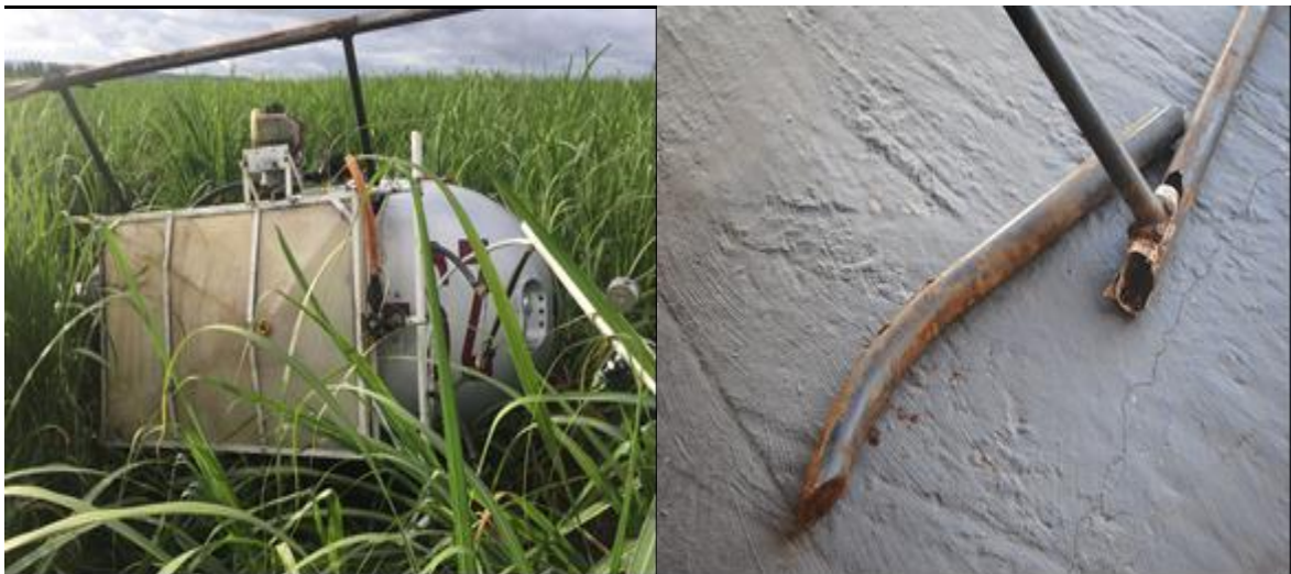
Figure 5: The position of the helicopter after the accident with broken skid
