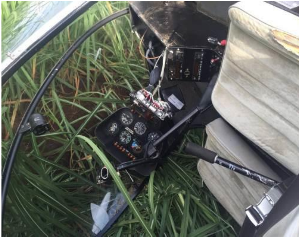
Figure 6: Damage to instrument panel
