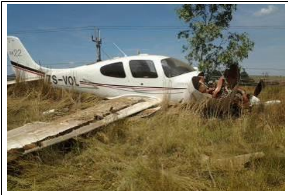
Figure 6: The front of the aircraft and the wings were badly damaged.
