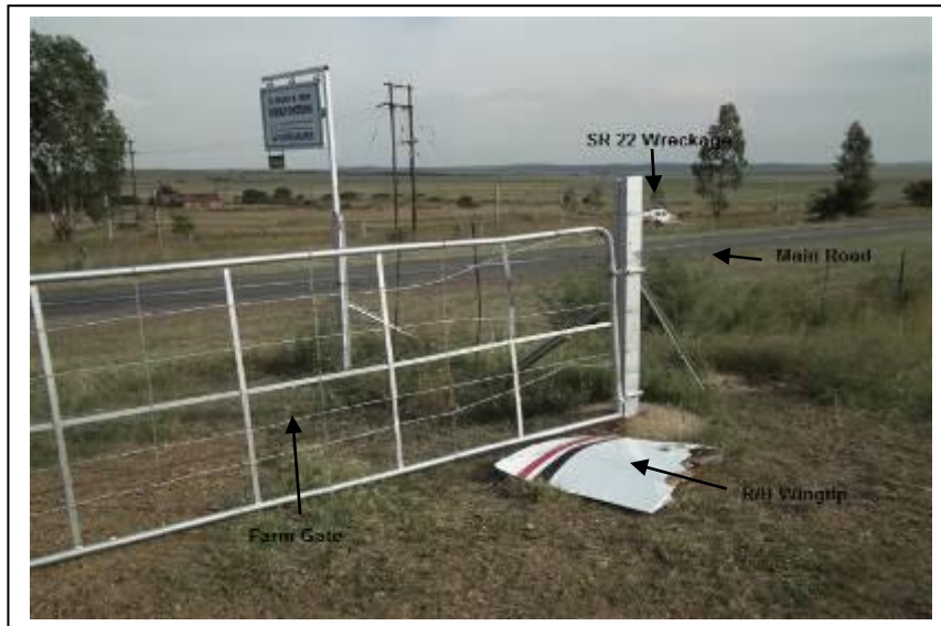
Figure 3: The left wing tip broke off after striking the gate.
