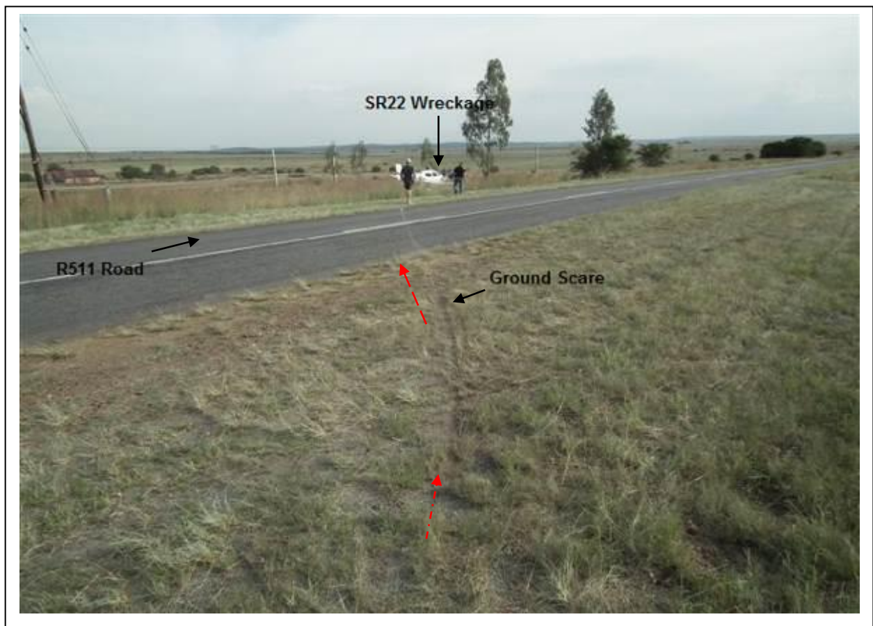
Figure 4: The ground marks produced by ZS-VOL as it skidded to a halt.
