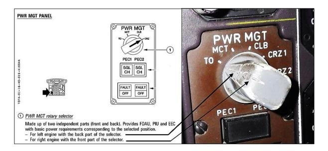
A Propeller Electronic Controller (PEC) controlled the commanded propeller rpm (NP). A Propeller valve module (PVM) would modify the propeller blade angle hydraulically by use of engine oil.
