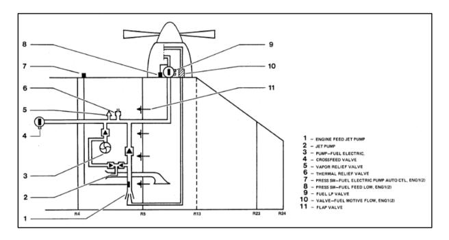
The electrical pump and the motive flow jet pump supplied the engine(s) during startup and operation.
