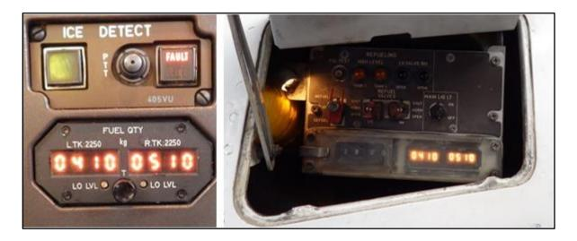
A "functional test of fuel quantity probe system" was performed in accordance with the aircraft manufacturer's JIC "28-42-72-FUT-10000-002".
