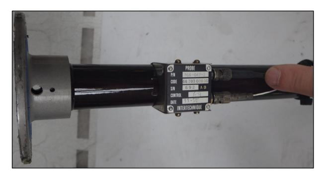
After further manipulation of the wire, the capacitance value of the probe returned to 36.7 pF which was within the limitation of the JIC. It was not possible to replicate the fault, and the faulty connector was replaced.
