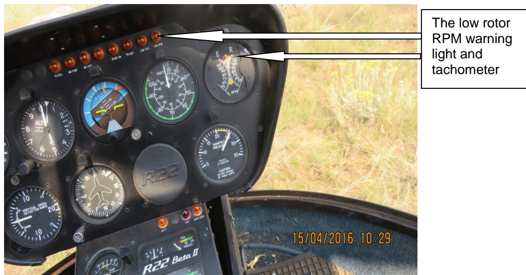
Figure 1: The helicopter’s low rotor RPM/blade stall warning light and the tachometer
