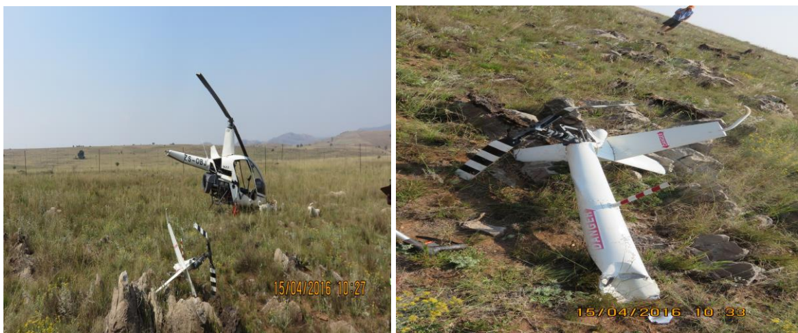
Figure 9: Photographs showing the wreckage lay-out and the closer shot of the tail rotor/fin
