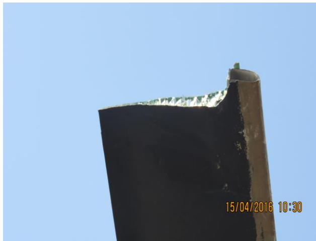
Figure 10: A photograph displaying of a severed rotor blade
