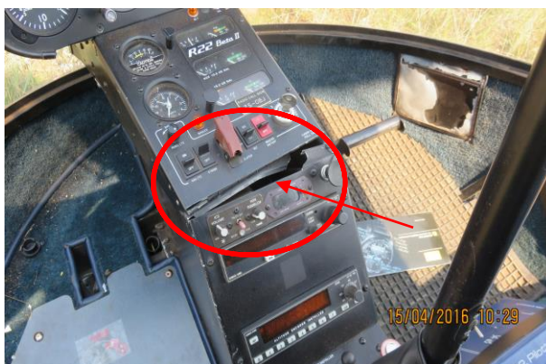
Figure 7: A photograph of a severed instrument panel
