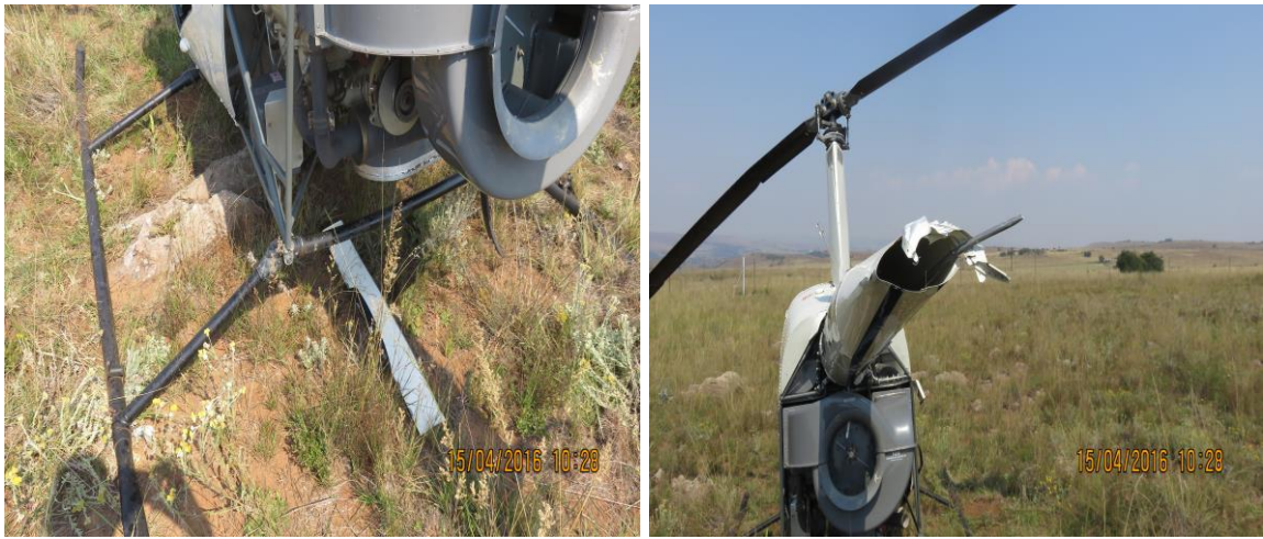
Figures 8: The skid gears as found (bowed out) and the severed tail boom
