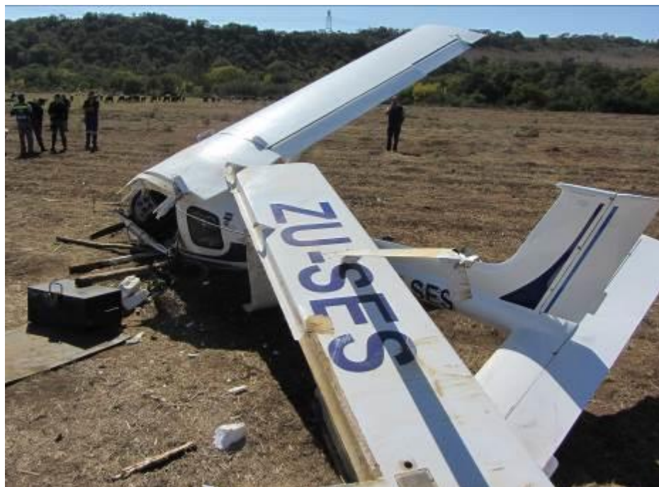
Figure 4 Damage to the left wing
