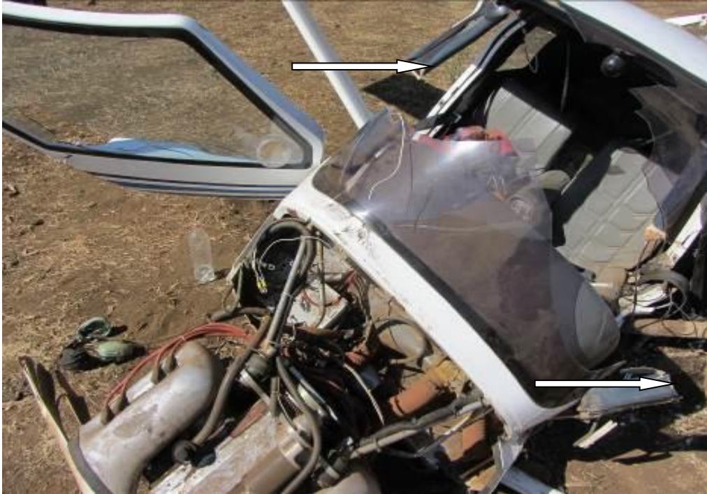
Figure 5 Broken window posts
