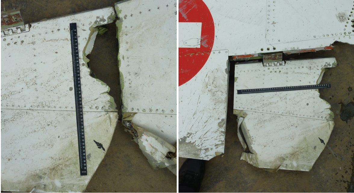
Figure 9: Two pieces of the left-hand aileron (left) and the left piece situated near its original place on the wing (right). (Source: Dutch Safety Board)
