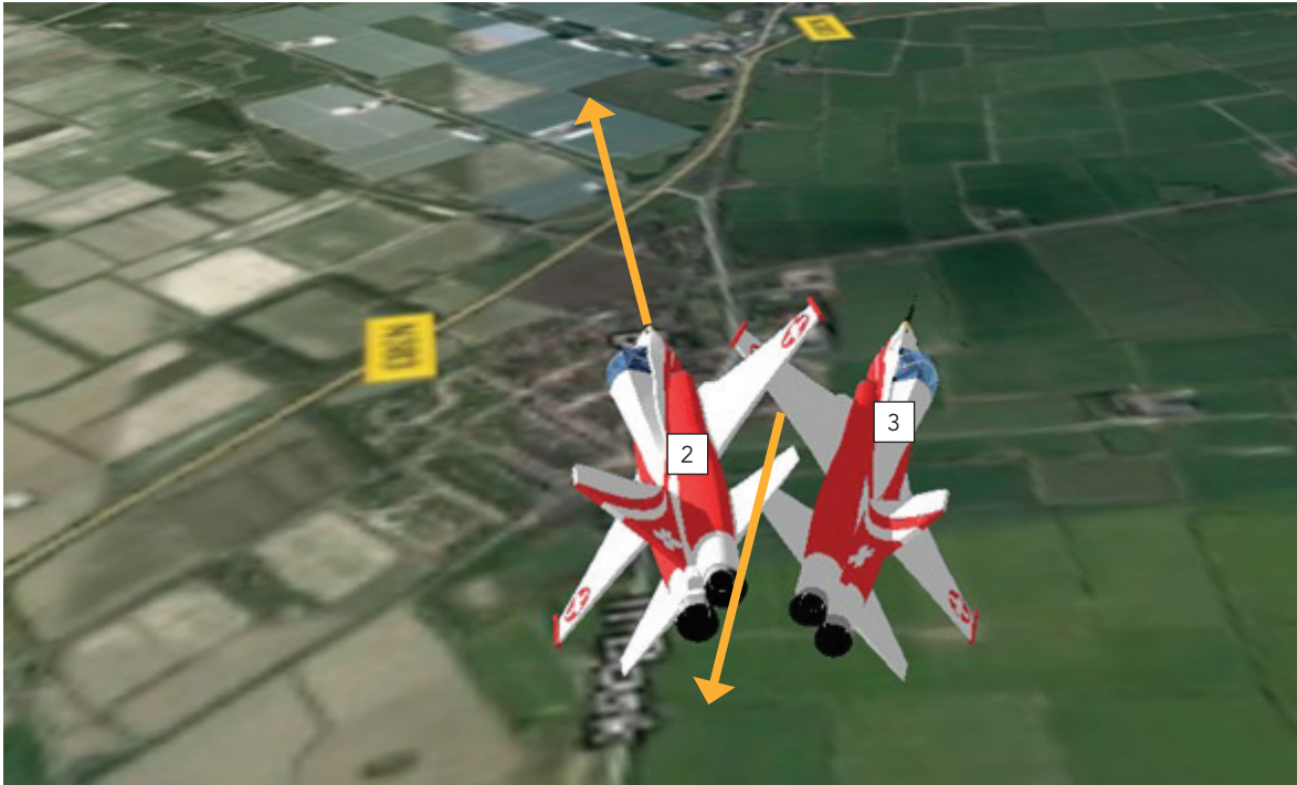
Figure 12: Estimated position and relative motion of aircraft numbers 2 and 3 at the time of the collision. (Source: Dutch Safety Board)
