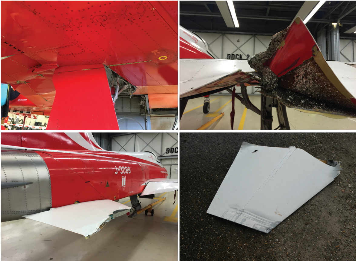
Figure 7: Damage of number 2 aircraft - underside right-hand wing (top left); right-hand trailing edge flap (top right); right-hand horizontal stabiliser (bottom left); found part of right-hand horizontal stabiliser (bottom right). (Source: Dutch Safety Board)
