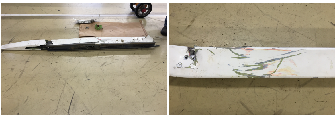
Figure 8: The number 3 aircraft left-hand missile launching rail. (Source: Dutch Safety Board)
