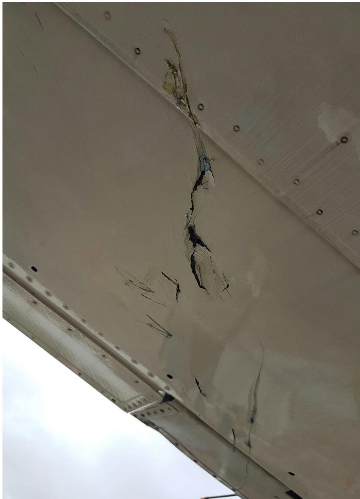
Figure : 5 The damaged lower skin of the RH Wing of the AT -72-212A (600 version) aircraft
