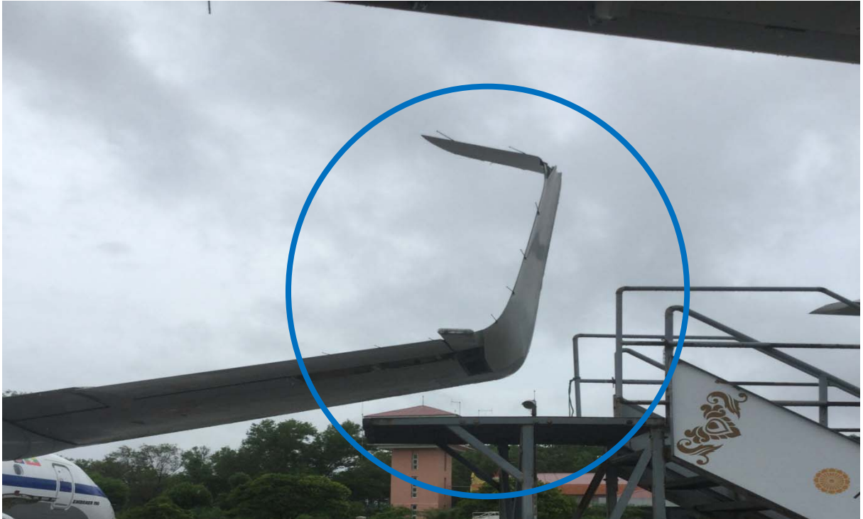
Figure: 8 The broke winglet of the RH Wing of the Embraer-190
