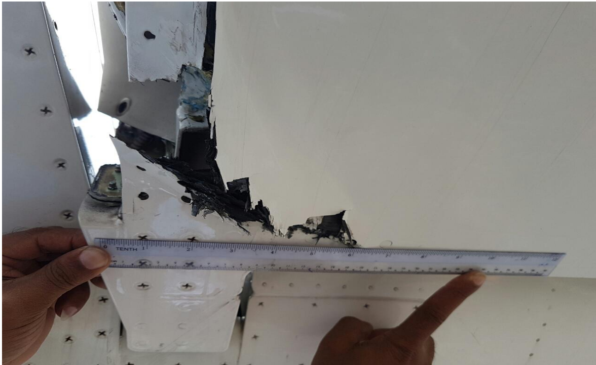
Figure: 6 The damaged lower skin of the RH Wing of ATR – 72-212A (600 version) aircraft
