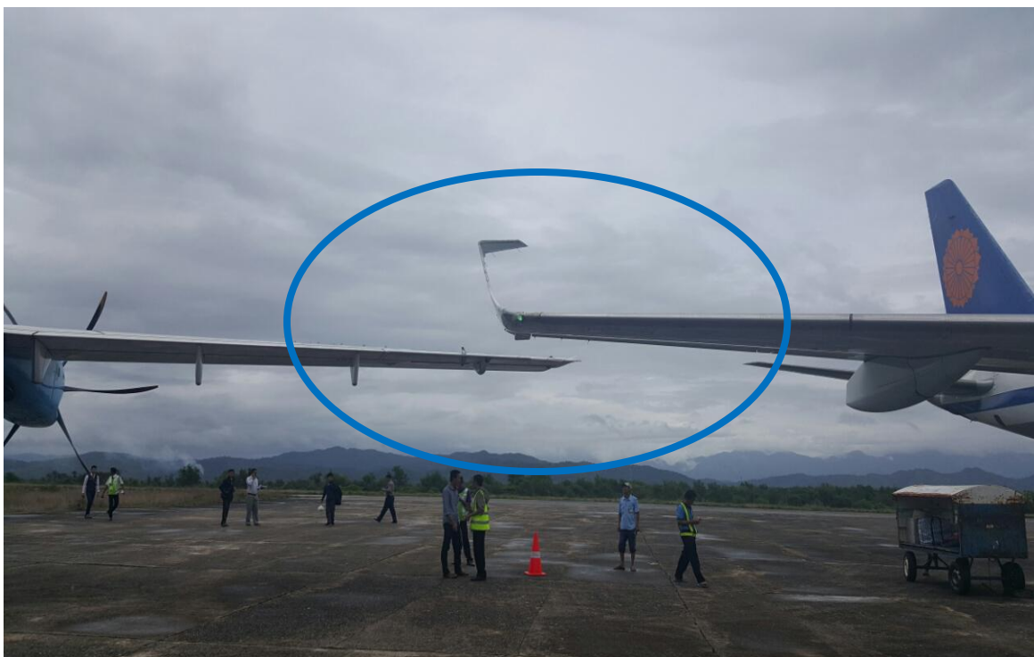
Figure: 3 Overview of damages to both aircraft
