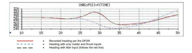
The trajectory shown with the blue dashed line is a simulation performed at Airbus using only the rudder pedal inputs and the engine thrust as recorded in the DFDR.
