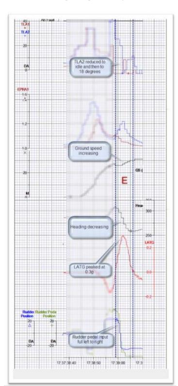
**17:38:54 UTC:** At 22kt (GS) increasing, while A/C was turning to the right, a left rudder pedal order was applied up to +38.9°.
