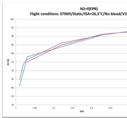
Considering the sampling, the use of the stabilized model in transient phase and the engine to engine variability, both engines are consistent with the model, showing no abnormal behavior.
