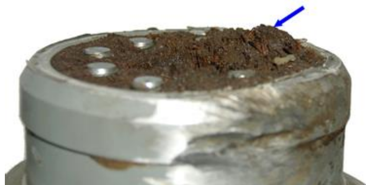
Fig. 21 Side view of one of the fracture areas of the broken-off bottom part of the propeller blade.
