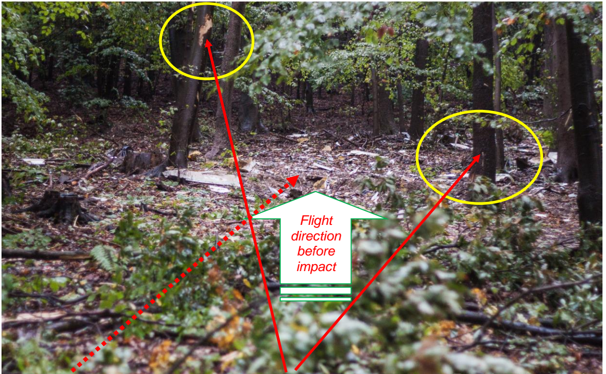
Fig. 15 Location of the engine and traces of wings before impact with the terrain - incline about 35°
