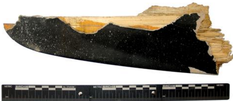
Fig. 24 Fragment of the propeller blade submitted as evidence No. 2
