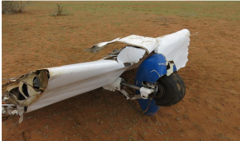
Figure 2: Shows the left-hand wing that separated from the a/c
