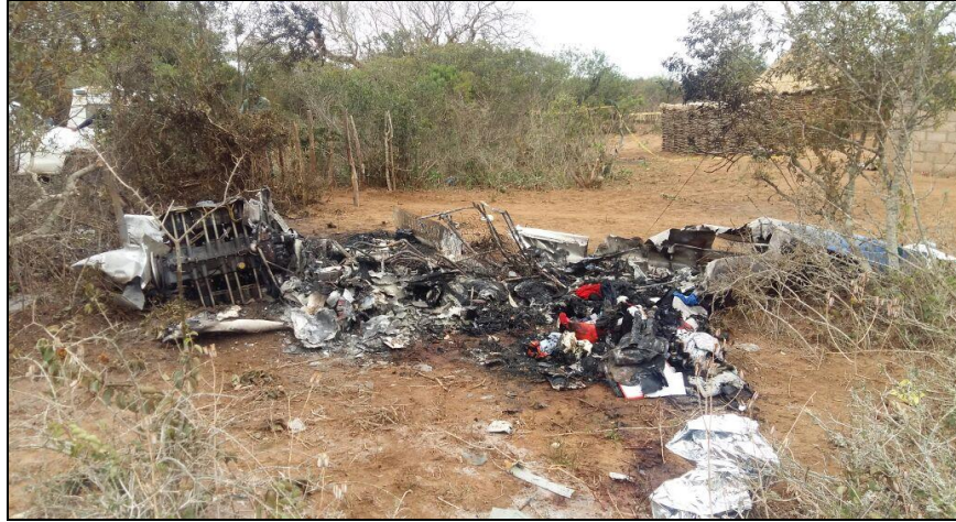
Figure 1: Wreckage of the aircraft destroyed by impact and post-impact fire
