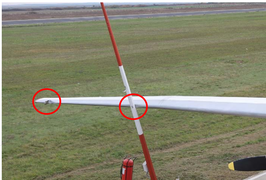
Fig.3 Aircraft wing damages
