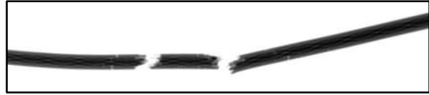
Figure 10. Tomography of wire No 3233-522 DR18 pin 4 5GF2A [Source: Airbus]
