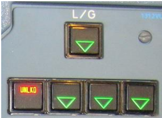
Figure 5. Left wing landing gear not down and locked
