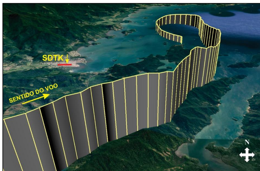
Figure 49 - Reconstruction of the descent profile of the aircraft, according to the RADAR air traffic control data.
