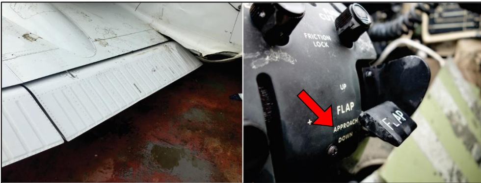
Figure 29 - Position of flaps and control lever (red arrow).
