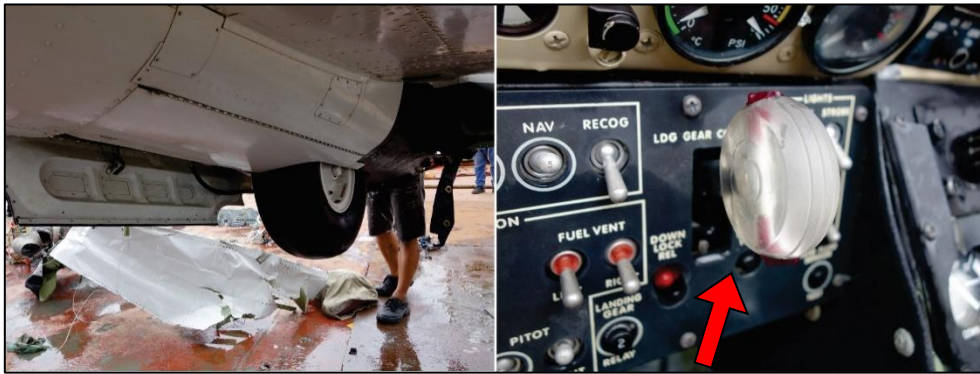
Figure 28 - Left landing gear positions and the control lever (red arrow).
