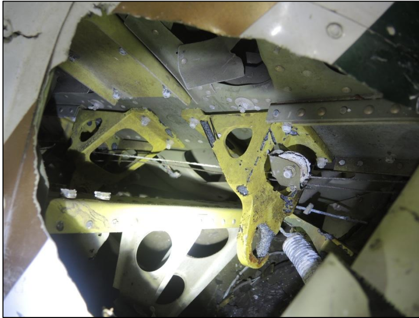
Figure 42 - Elevator control cables.
