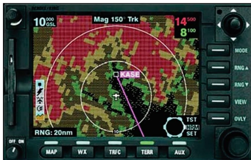
Figure 5 - MFD of the same model of the PR-SOM aircraft, selected in terrain mode, and displaying the EGPWS information.
