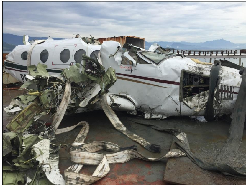
Figure 26 - Right side view of the aircraft after its removal from the sea.
