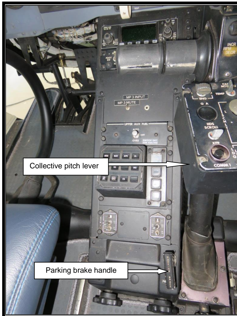
Figure 15: The parking brake handle next to the collective pitch lever
