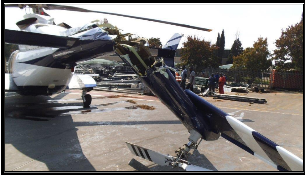
Figure 7: The severed tail boom structure.
