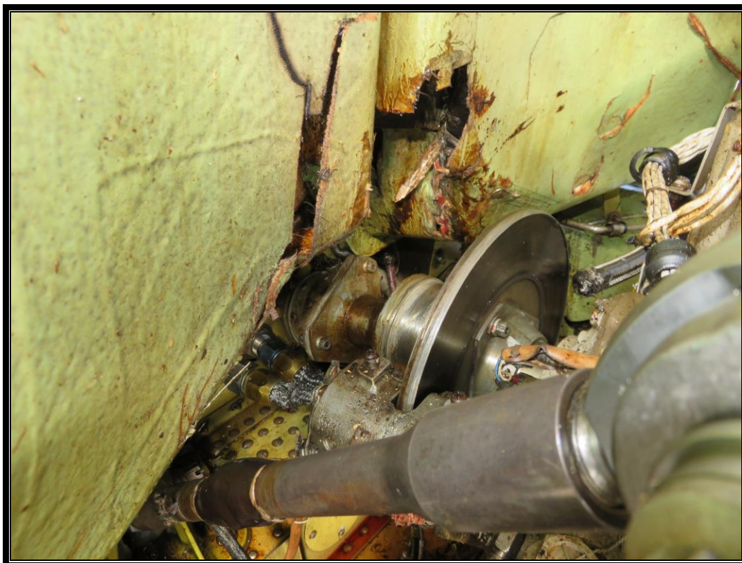
Figure 11: Damage caused by tail rotor drive shaft that failed aft of the rotor brake assembly.
