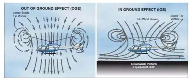
When the helicopter is near the ground, this vertical component of air from the main rotor impacts with a hard surface (the ground), and give a
