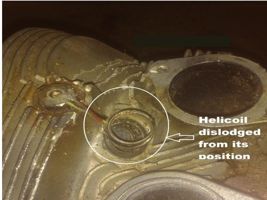
Fig:19: Dislodged Helicoil
