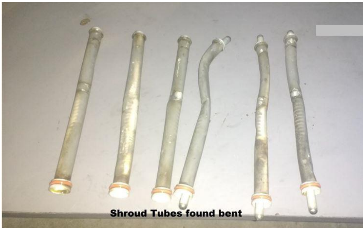
Fig: 35: Bend shroud tubes
