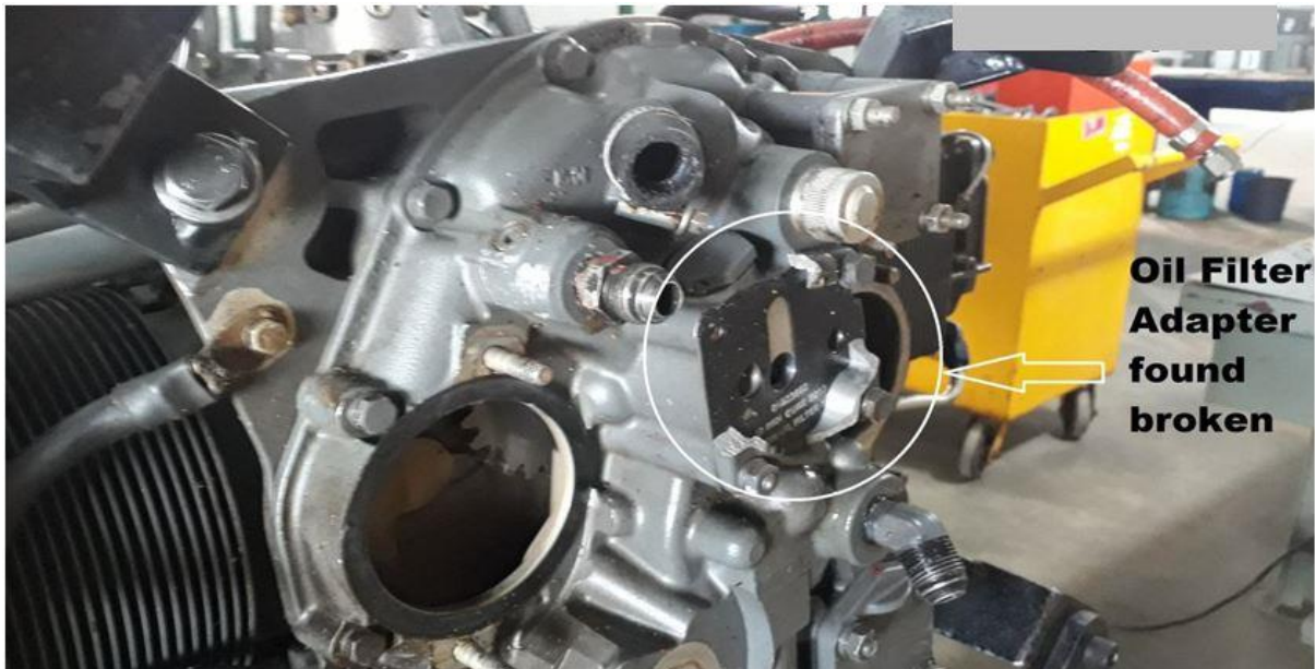
Fig: 26: Broken oil filter adapter
