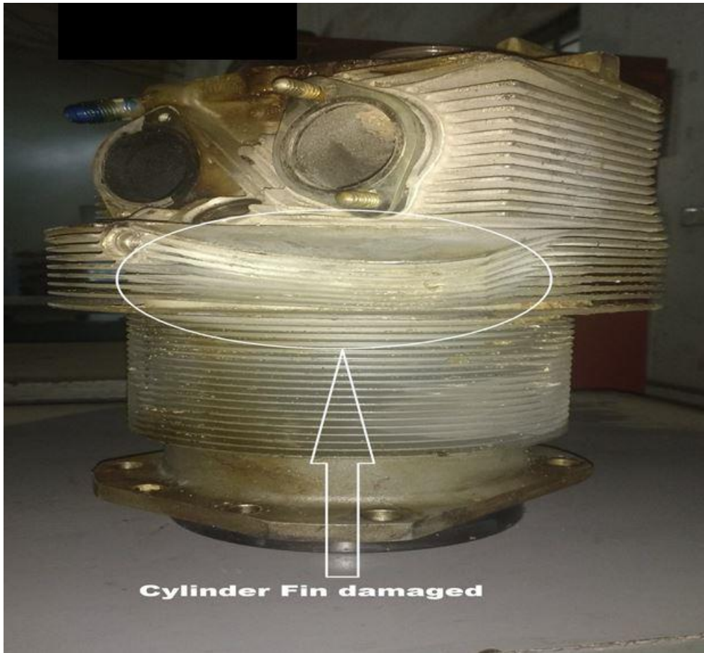
Fig: 28: Damaged Cylinder Fin
