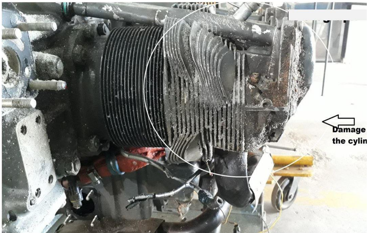
Fig: 18: Damaged Cylinder
