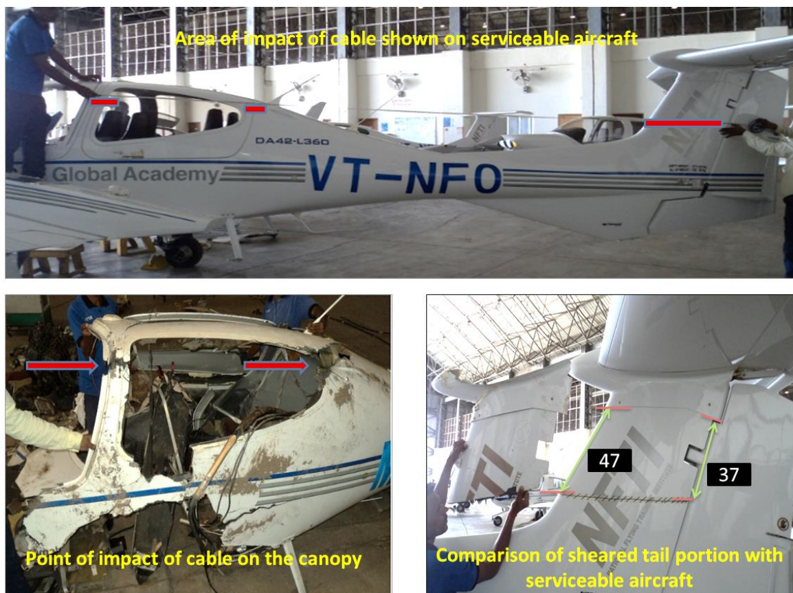
Fig 15: Comparison of wreckage with serviceable aircraft
