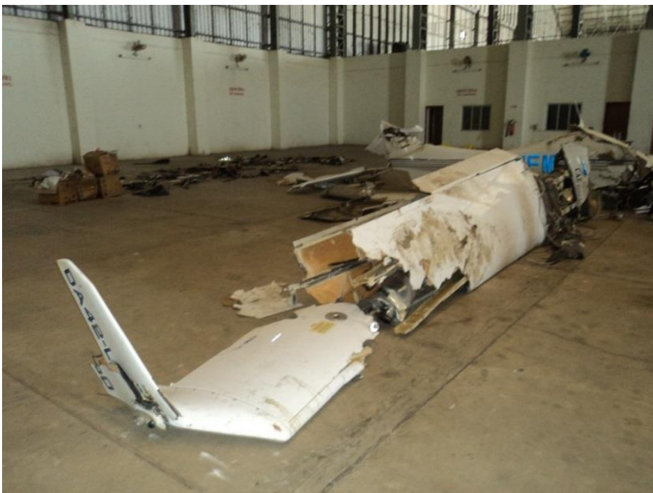
Fig 9: RH wing wreckage after layout
