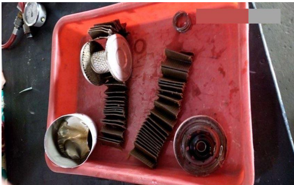
Fig: 33: Oil filter cut for inspection
