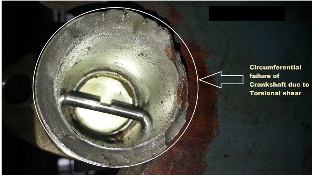
Fig: 23: Failed crankshaft
