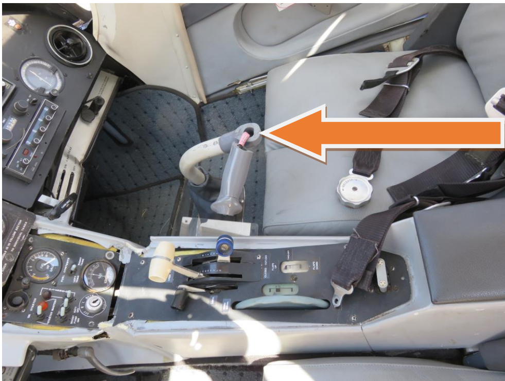
Figure 7: Arrow shows a view of the broken control grip on the navigator side.
