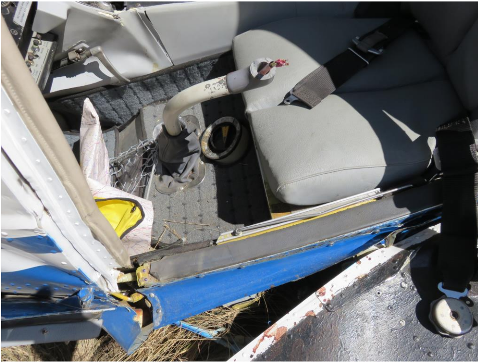
Figure 8: A view of the broken control grip on the pilot side
