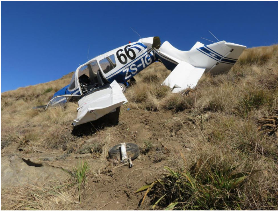
Figure 4: Side view of the wreckage as it came to rest, nose gear broken off
