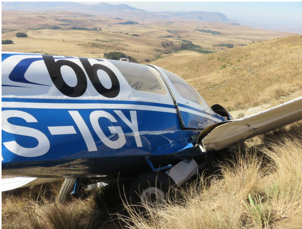
Figure 6: A view of the main landing gear that collapsed and folded backwards
