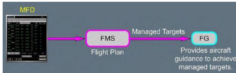
Figure 10. Managed guidance [Source: Airbus]
