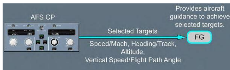
Figure 9. Selected guidance [Source: Airbus]
