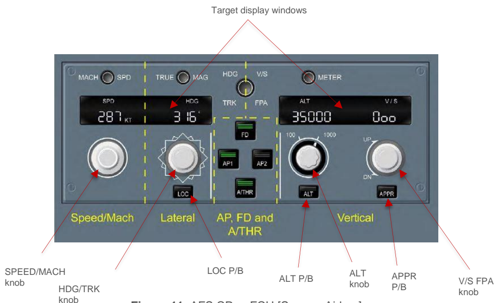
Figure 11. AFS CP or FCU [Source: Airbus]
