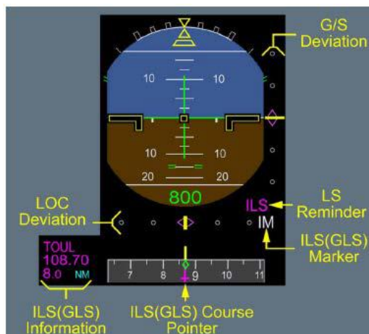
Figure 19. ILS information on PFD [Source: Airbus]
