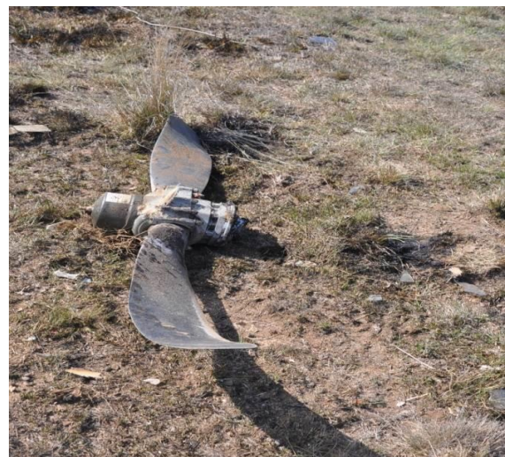
Figure 7/8: Pictures showing a broken engine crankshaft (L) and the propeller (R)
