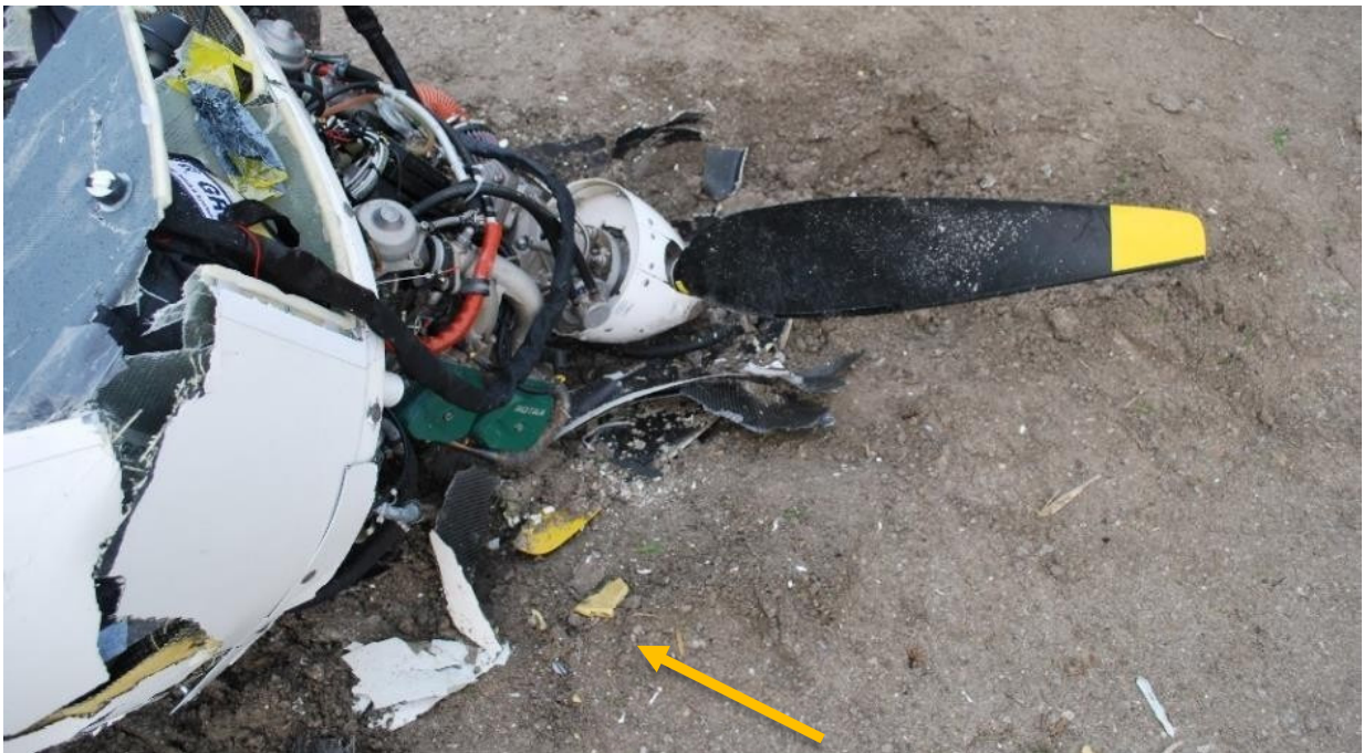
A propeller blade is severed at impact and is subsequently located under the aircraft on the starboard side (underneath the co-pilots rudder pedals). The second blade remains intact and attached to the propeller hub, pointing to starboard relative to the aircraft.
