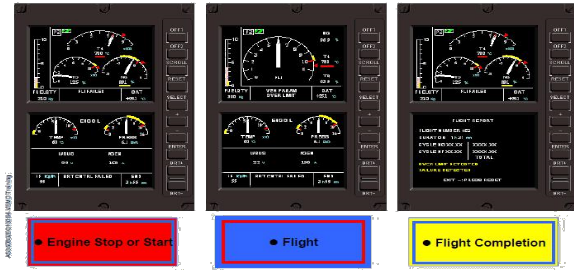
Figure 6; Graphs showing Central Panel Display System (CPDS) phases of operation.
