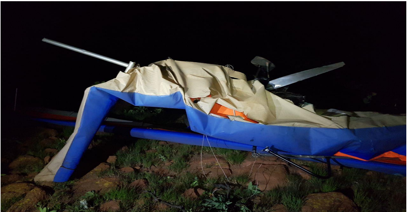
Figure 4: Damage to the left-hand side of the wing
