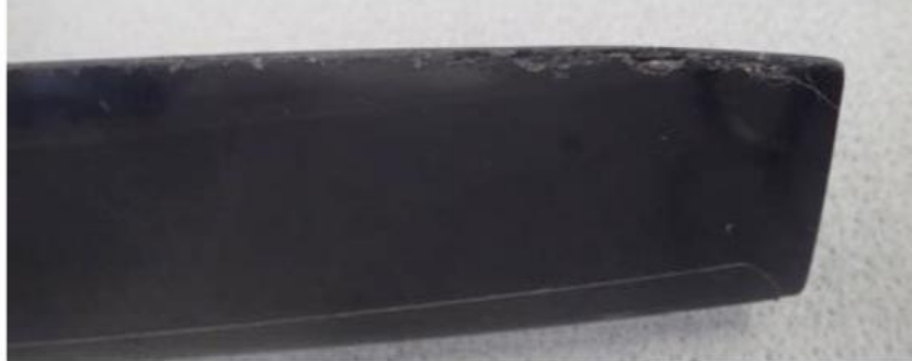
Figure 17: extremity of blade with damage on the trailing edge
