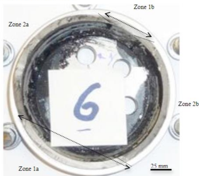
Figure 6: fracture surface of the fixation ring of propeller blade 2; indication of particular zones. Zones 1a and 1b correspond to the propagation of a fatigue crack; zones 2a and 2b correspond to the overload fracture of the ring. For further explanation, see text.
