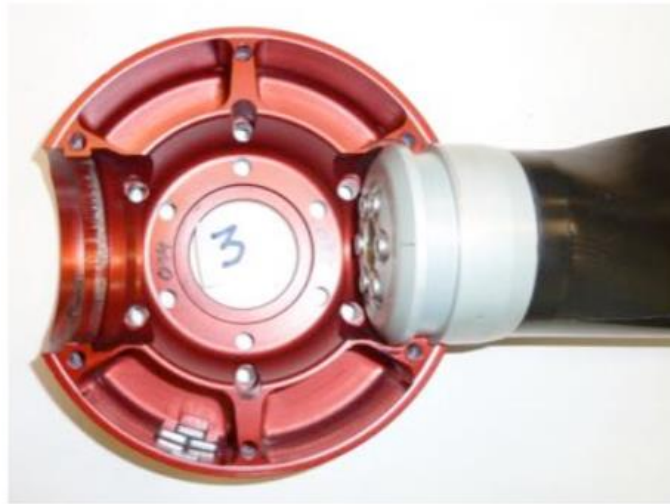
Figure 15: overview on a hub half with the undamaged propeller blade in place
