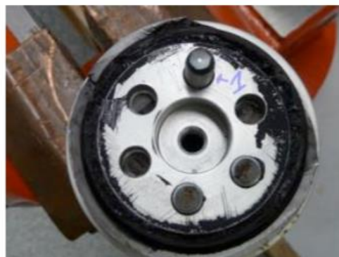
Figure 4: fragment of the fixation ring that remained fixed to the propeller blade (lower part on figure 3); fragments from the broken bolts are still present in the bore holes. Bolt 1 is identified with blue marker. The black material between the outer remnants of the fixation ring and the inner metallic insert are the carbon fibre/resin composite material.
