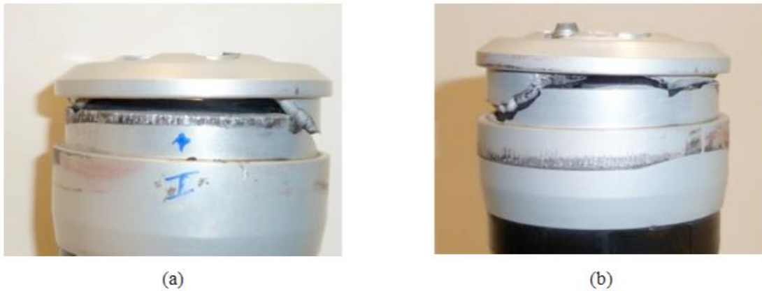
Figure 3: both complementary parts of the fractured fixation ring have been put together; they exhibit perfectly axial surface grooves caused by centrifugal projection of the blade after primary failure of the fixation ring
