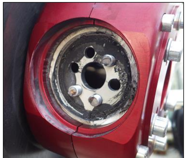
Figure 9 : zoom on the damage of the hub
