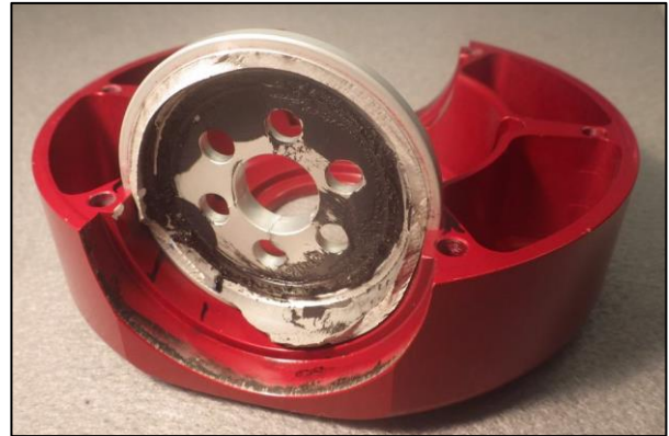
Figure 11 : broken part of the blade root left in the hub
