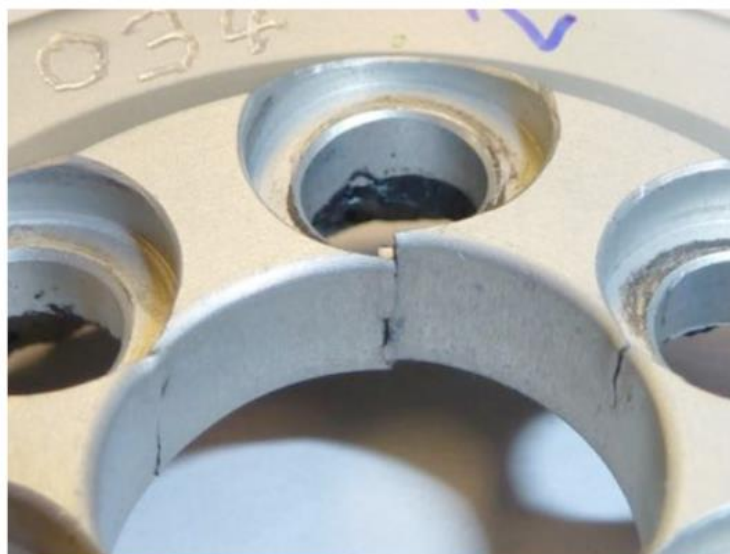
Figure 11: detail of the crack near hole No. 1, as indicated on figure 10
