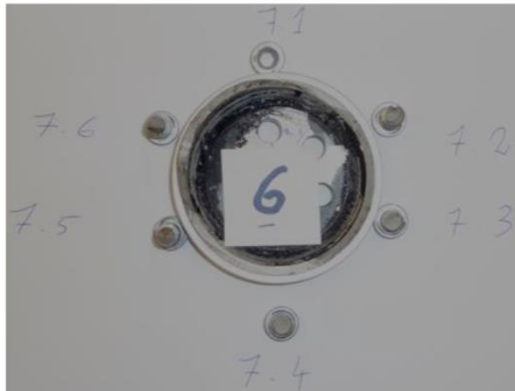
Figure 5: complementary part of the fixation ring (upper part on figure 3), together with the fragments of the broken bolts (see also figure 4). Bolt fragments have been numbered for detailed analysis
