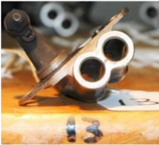
Figure 2 Typical fuel nozzle condition as received
