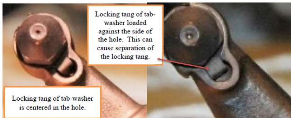
Figure 3 Nozzle tip tab washer correctly applied (left) and incorrectly applied (right).
