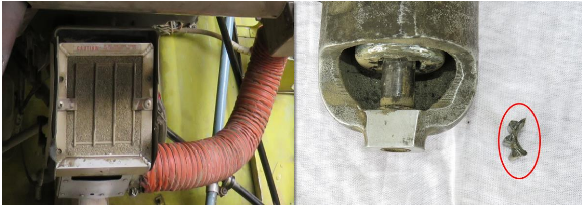
Fig 12: Air intake filter and broken piece of starter gear
