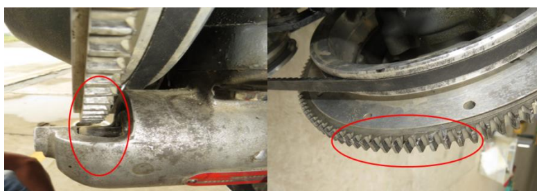
Fig 11: Broken Starter Gear and Ring Gear teeth
