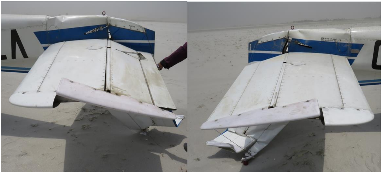
Fig 5: Damages to Tail Fin and Tail Cone
