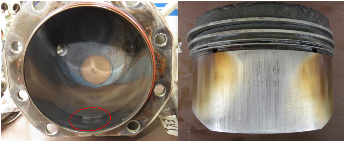
Fig 14: Scoring marks on Cylinder No 1 and its Piston
