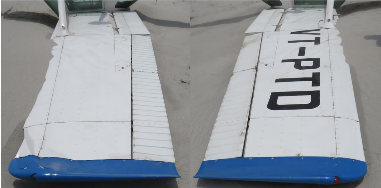
Fig 4: Damages to LH and RH wing
