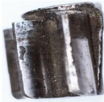
Fig 20: Pitting on the gear
