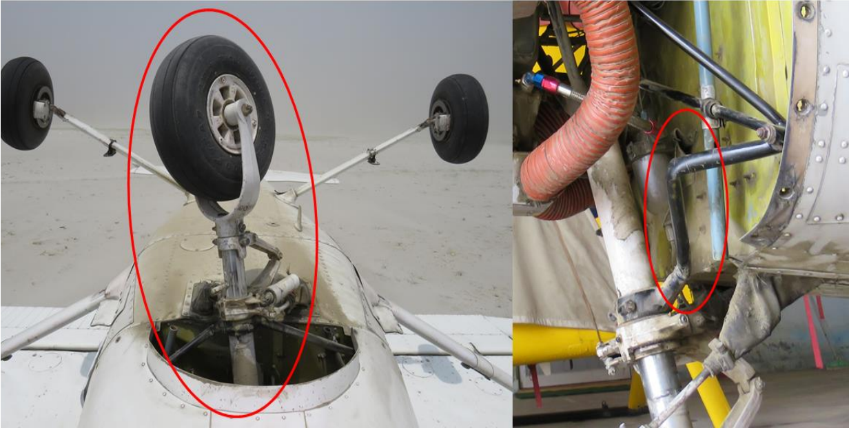
Fig 2: Nose Landing gear bent due to bending of its mounting
