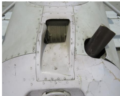
Fig 10: Damage to the nose cowling and exhaust stag
