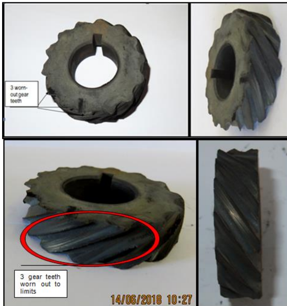
Figure 7 : Shows the worn out distributor driving gear teeth
