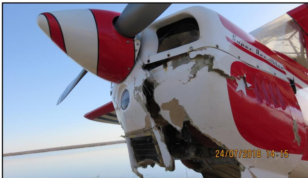
Figure 3: Damaged bottom engine cowlings
