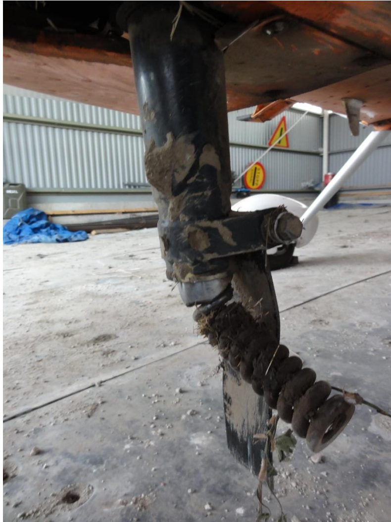
Figure 8. The top part of the nose landing gear.
