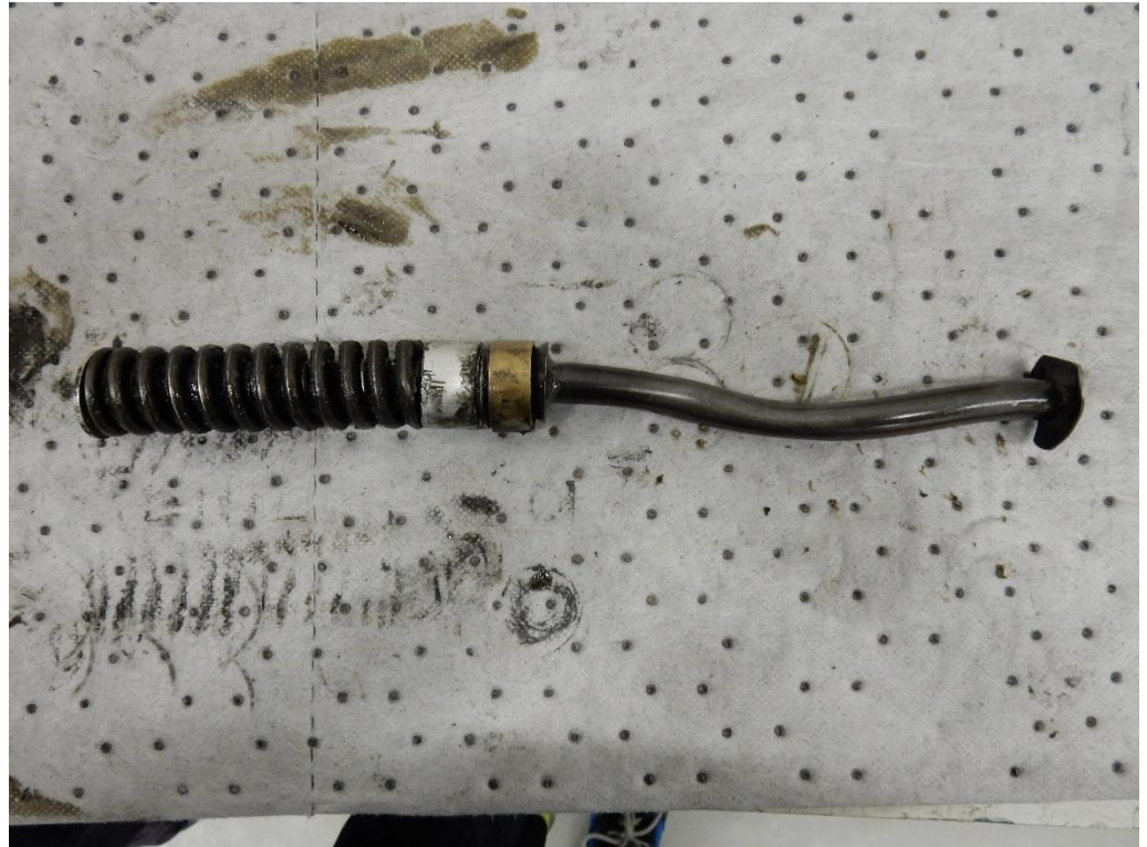
Figure 9. Part of the spring assembly and the deformed metal rod.
