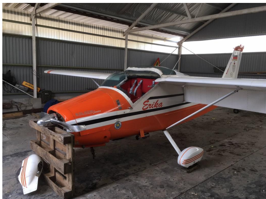
Figure 6. The wreckage after being towed to the hangar.
