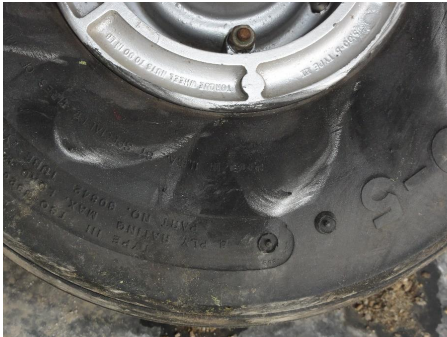
Figure 7. Traces of paint from the wheel fairing on the tyre.
