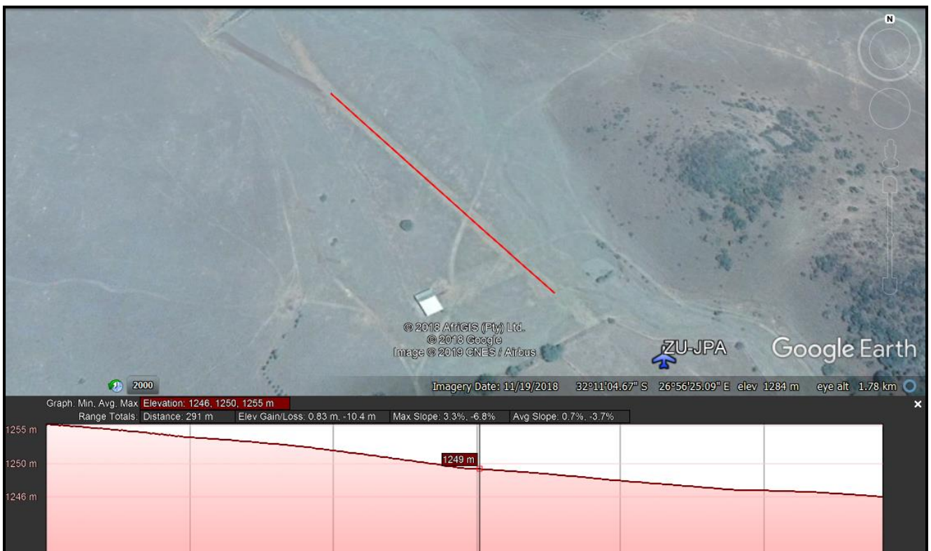
Figure 1: Runway 14 has a downward slope at an average of 3.7% and is 290m (951 feet) long.
