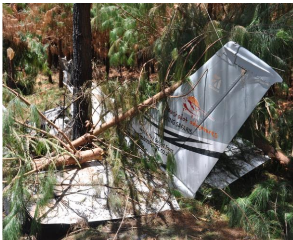
Figure 7: The aircraft tail section after the accident.
