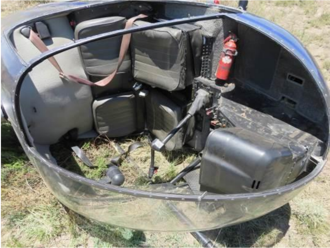
Figure 5: A view of the cockpit/cabin area, which remained intact apart from the left windshield that broke
