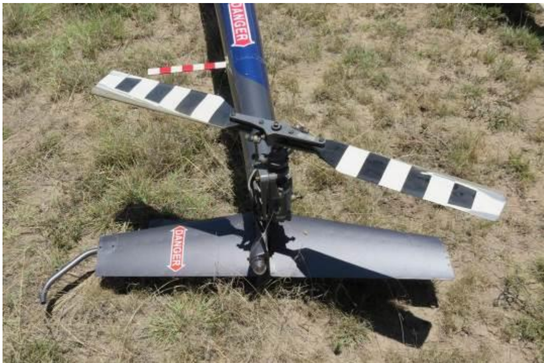
Figure 4: A view of the tail rotor assembly, which did not sustain any damage
