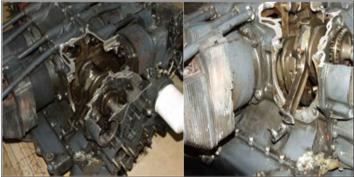
Figure 12 and 13 show similar failures from ATSB. An overview of the rear of the left engine after being removed from the aircraft; and the fractured small end of the No. 6 connecting rod.
