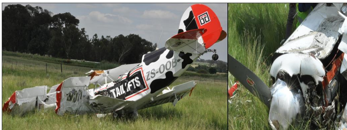
Figure 3: Damages on the aircraft's left side, engine compartment and propeller spinner.
