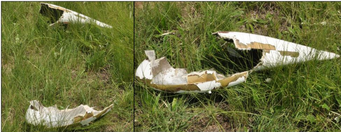
Figure 4: The detached left main landing gear wheel fairings covers.
