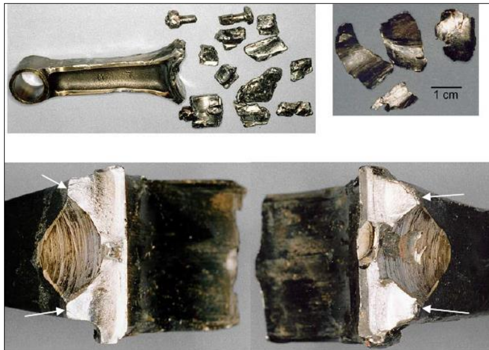
Figure 10: The recovered fragments of the big-end housing (top left), some of the larger fragments of the bearing inserts (top right), detailed view of both housing fractures at the transition to the rod “I” beam (bottom). The sites of fatigue initiation are arrowed. [Source: ATSB’s Analysis of Aircraft Reciprocating-Engine Failure, pg.63]
