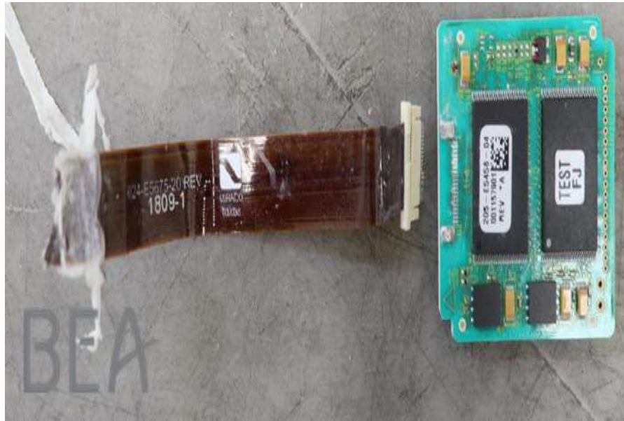
FIGURE 34: FDR MEMORY BOARD, FLEX AND CONNECTOR
