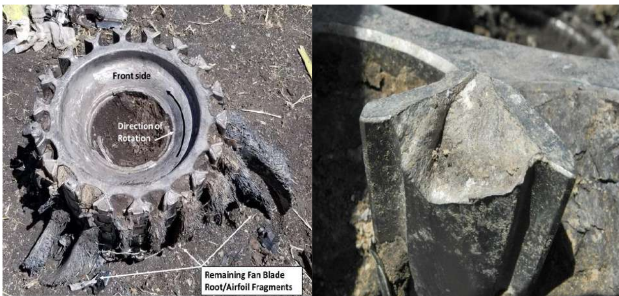
FIGURE46: R/H ENGINE - S/N 602695 - FAN DISK FIGURE47: R/H ENGINE - S/N 602695 - RETENTION LUGS - FRACTURED
