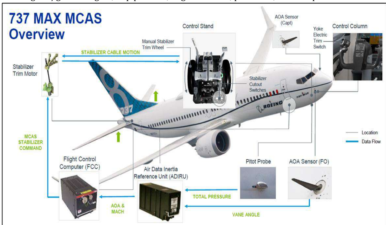
FIGURE 20: DIAGRAM SHOWING THE COMPONENTS OF MCAS 16
