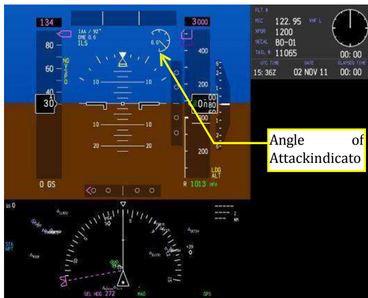
Figure10:AOA Indicator on PFD
