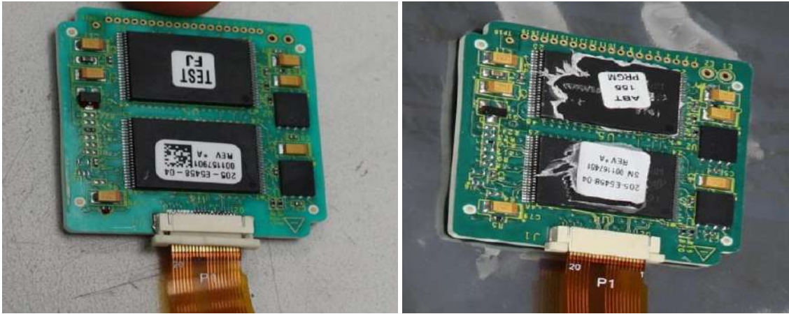
FIGURE 7: ET-AVJ FDR MEMORY BOARD WITH INTERFACE BOARD CONNECTOR FROM BEA SURROGATE RECORDER (LEFT), BEA SURROGATE RECORDER MEMORY BOARD WITH ORIGINAL CONNECTOR (RIGHT), BOTH MOUNTED WITH FLEX CABLE PIN VISIBLE AND "P1" WHEN PERFORMING READOUT
