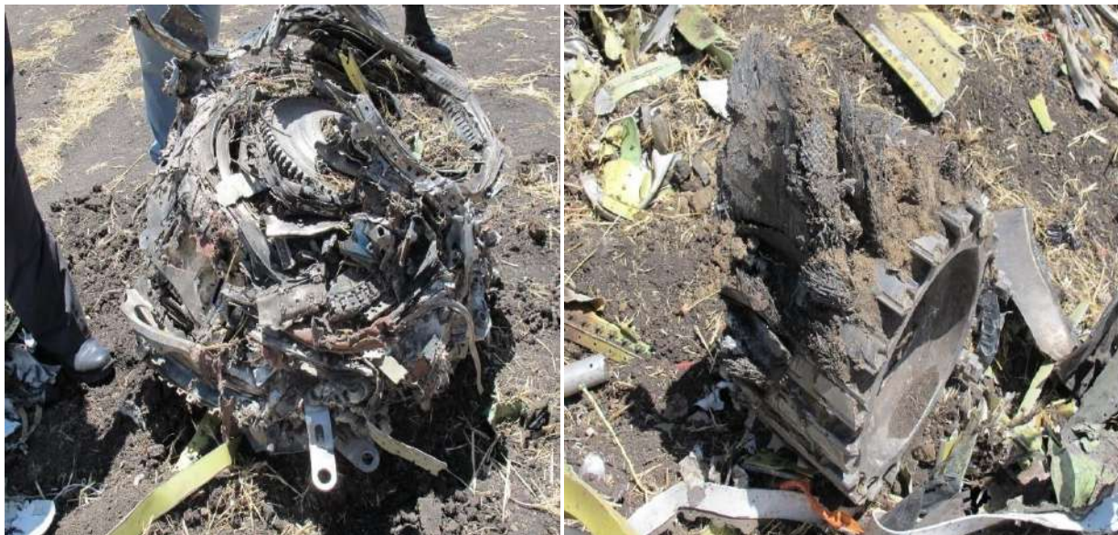
FIGURE 44: R/H ENGINE - S/N 602695 - CORE FIGURE 45: - R/H ENGINE - S/N 602695 - FAN DISK
