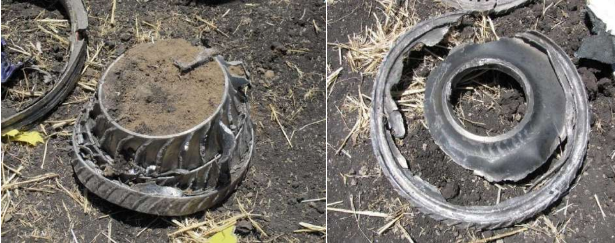
FIGURE 48: - R/H ENGINE - S/N 602695 - HPC STAGES 1 TO 3 FIGURES 49:- R/H ENGINE - S/N 602695 - HPC STAGE 7
