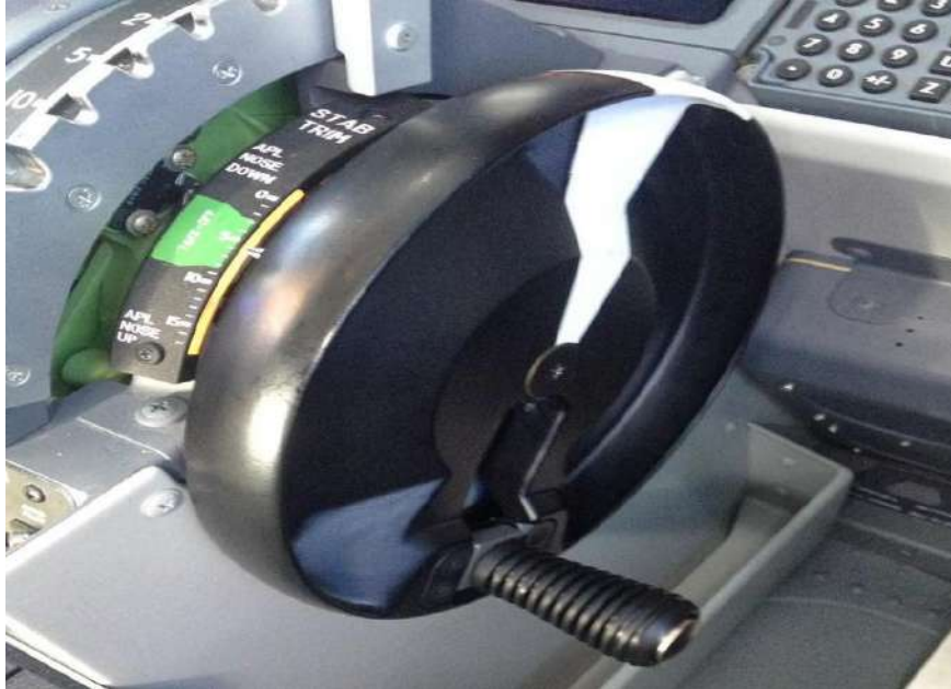
FIGURE 19: THE TRIM WHEEL, WITH THE HANDLE EXTENDED
