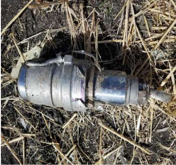
FIGURE 57: SLAT ACTUATOR (POSITION UNKNOWN)
