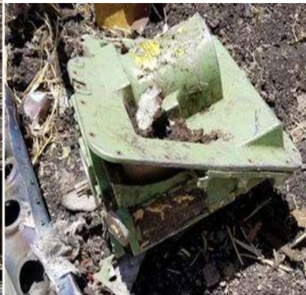
FIGURE60: STAB TRIM ELECTRIC MOTOR HOUSING
