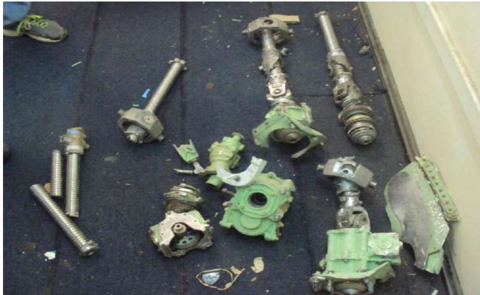
FIGURE56: TRAILING EDGE FLAP TRANSMISSIONS AND BALL SCREWS
