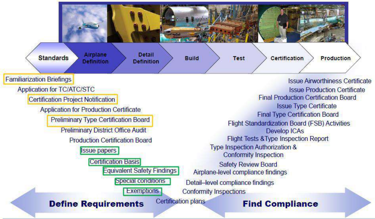
FIGURE 90: DIAGRAM OF FAA CERTIFICATION PROCESS
