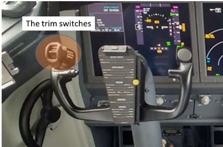
FIGURE 18: TRIM SWITCHES ON THE LH YOKE
