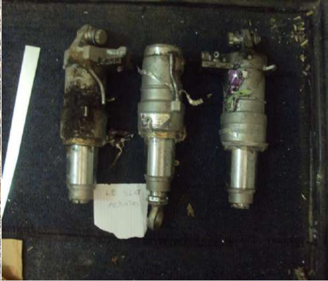
FIGURE 58: LEADING EDGE SLAT ACTUATORS
