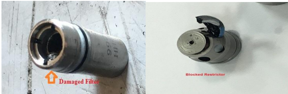
Failed Check Valve
