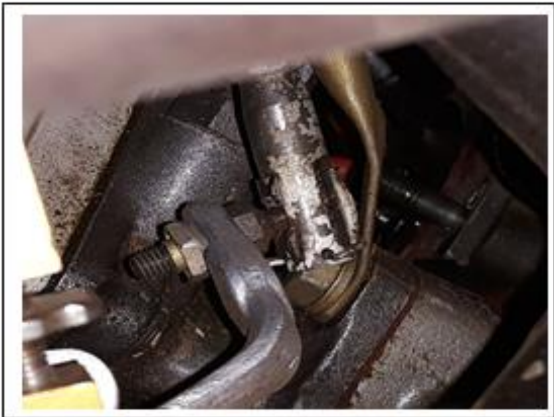
Figure 8: The ball joint retainer that was removed by the investigating team.
