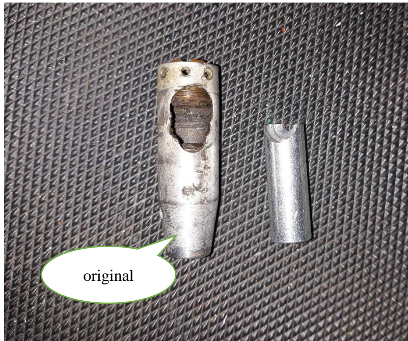
Figure 9: The difference between the manufacturer-approved cable end fitting (original) and the unapproved cable end fitting that had failed.
