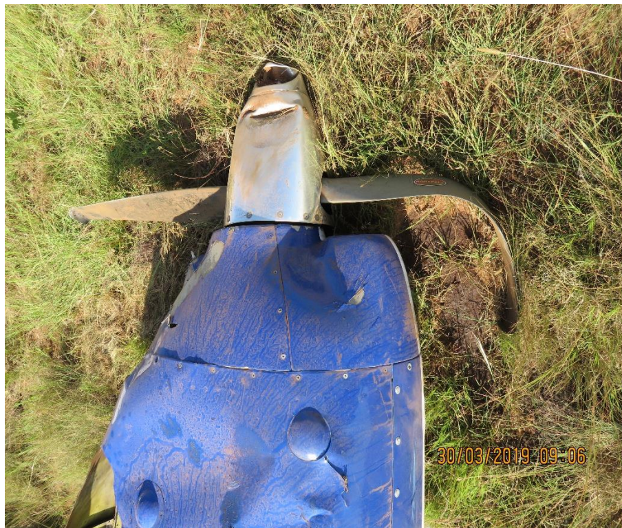
Figure 3: The damaged right-side engine propeller.
