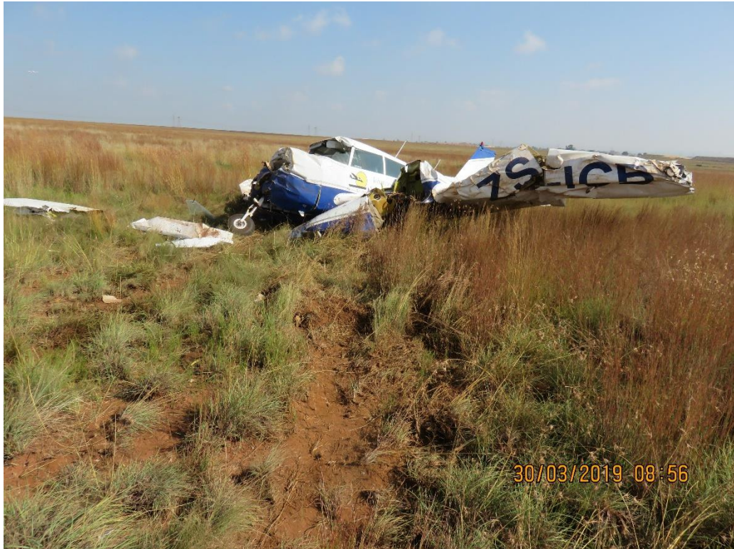
Figure 5: The skid marks on the ground and the broken off right-side outboard wing.
