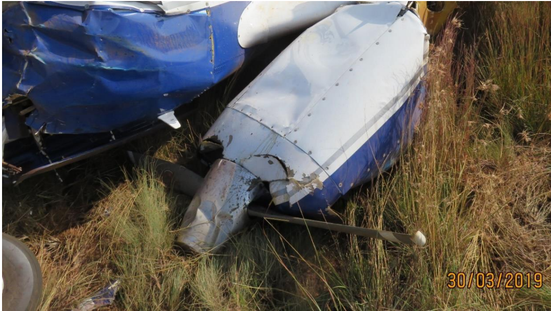
Figure 4: The left-side engine propeller with tips bending backwards. Both propellers were rotating at different revolutions per minute (RPM).
