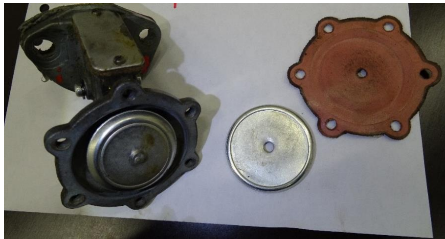
Figure 14. Part of the fuel pump with the loose drive plate and the diaphragm.
