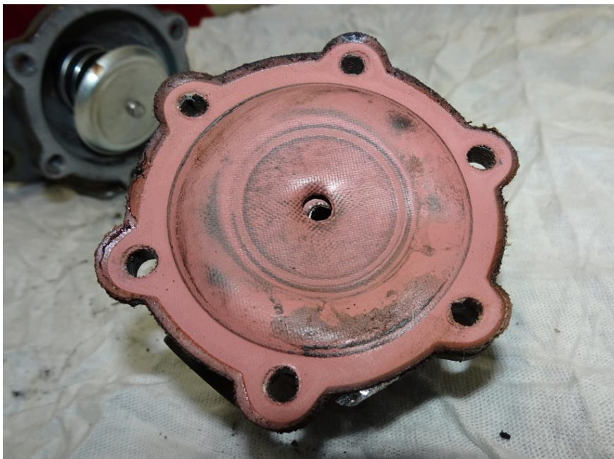
Figure 12. In the foreground in the image is the diaphragm with the outer half of the fuel pump housing. In the background is the other half of the fuel pump housing with one of the plates that drives the diaphragm.
