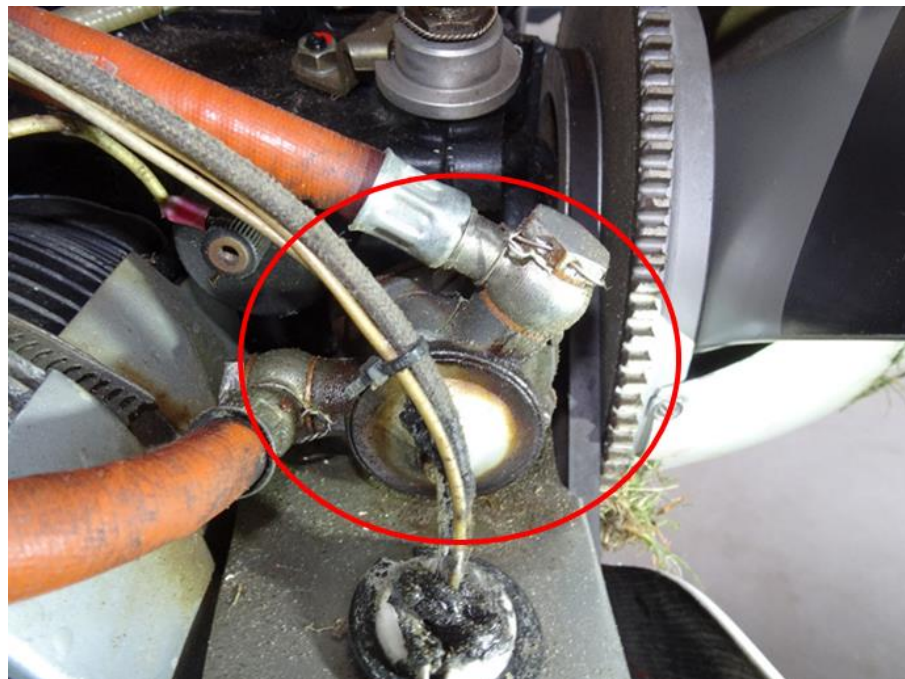
Figure 3. Mechanical fuel pump mounted on the engine, manufactured by APG.
