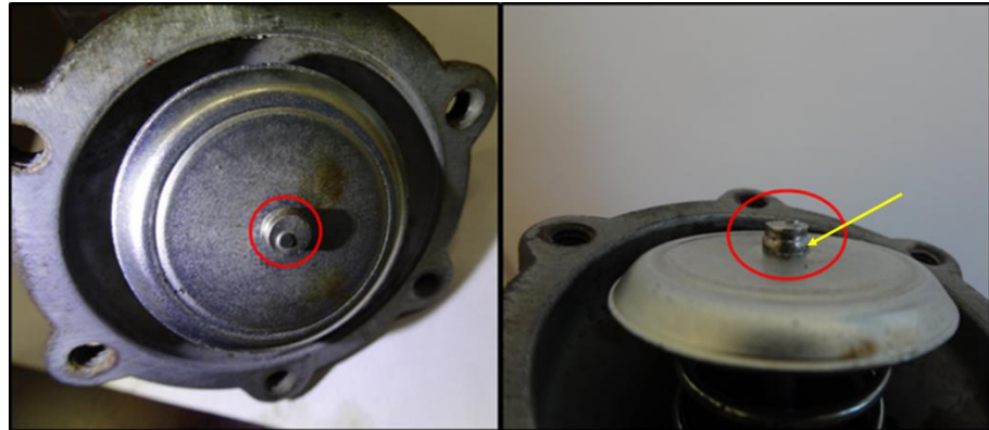
Figure 13. The image shows the interior plate, which is part of how the diaphragm is driven. In the middle of the plate is the part that is supposed to hold the plates and the diaphragm together, the shank and the formed head (the rivet head). The right image shows the swelled shank, marked with a yellow arrow.
