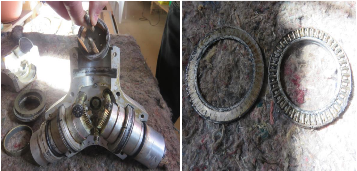
Figures 5 & 6: On the left is a dismantled propeller hub with some of the bearings visible, and on the right are the main bearings.
