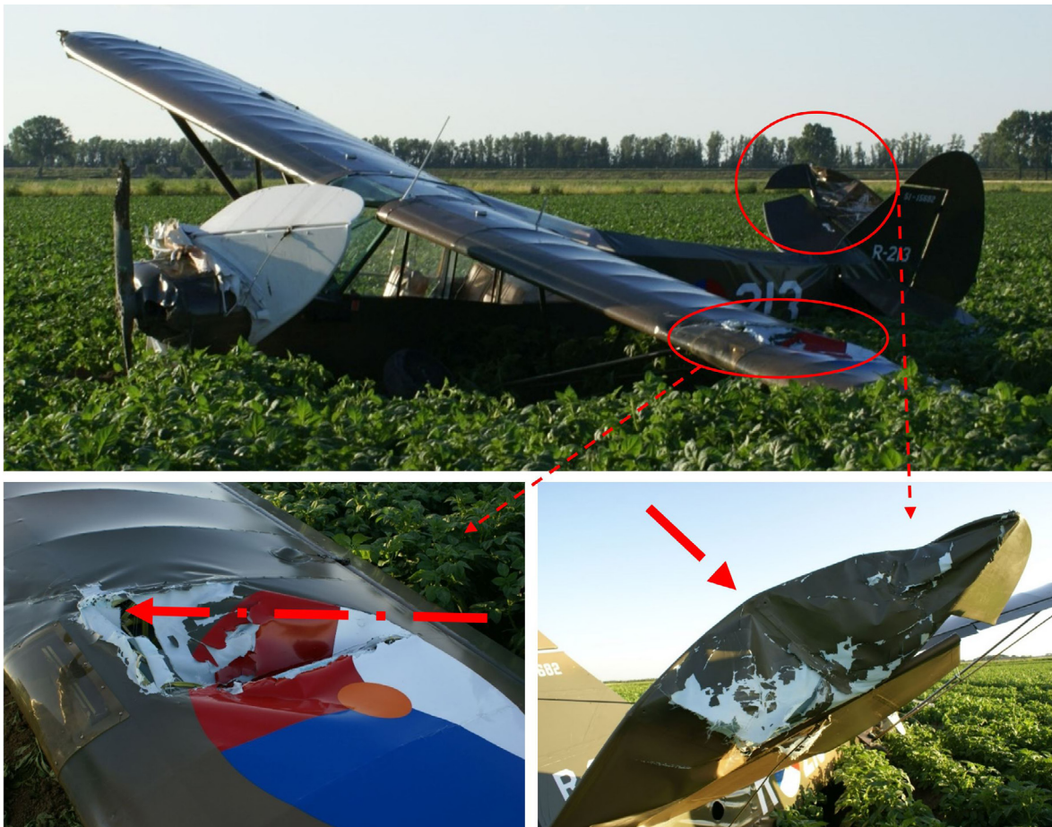
Figure 2: PH-RED's damage pattern right elevator and left wing tip. (Source: Dutch Safety Board)
