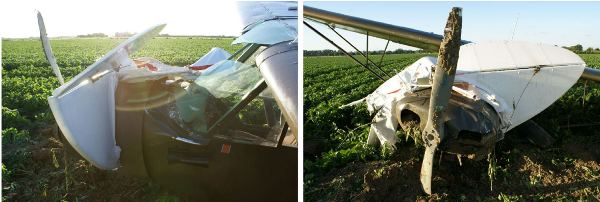
Figure 3: PH-RED's damaged windscreen and PH-VCY's horizontal stabiliser blocking PH-RED's windscreen. (Source: Dutch Safety Board)
