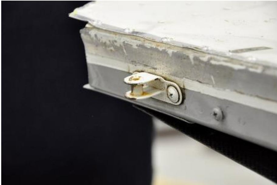
Figure 57. The cabin door's locking pin on the fuselage.
