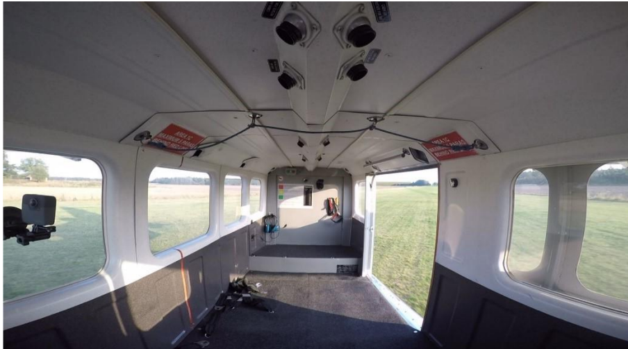
Figure 10. Picture of the cabin taken from the cockpit of another aeroplane of the same type. SE-MES was not equipped in the same way as the aeroplane in the picture, there were no safety belts or ropes on the ceiling to hold on to. According to the type certificate holder, the raised section of the floor ( the baggage shelf ) furthest back may not be used when parachute operations are conducted.
