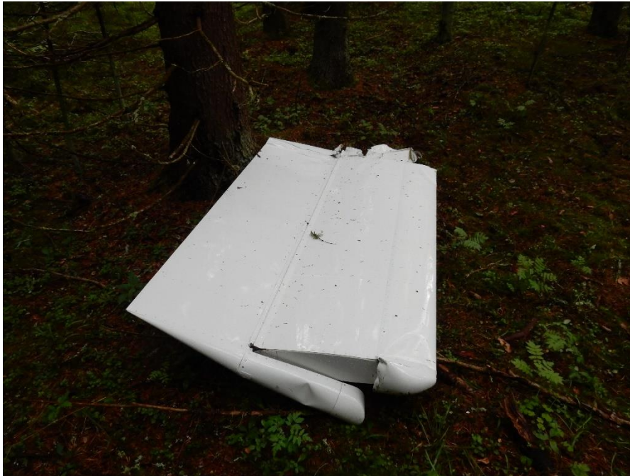
Figure 30. The broken part of the left side of the stabiliser.
