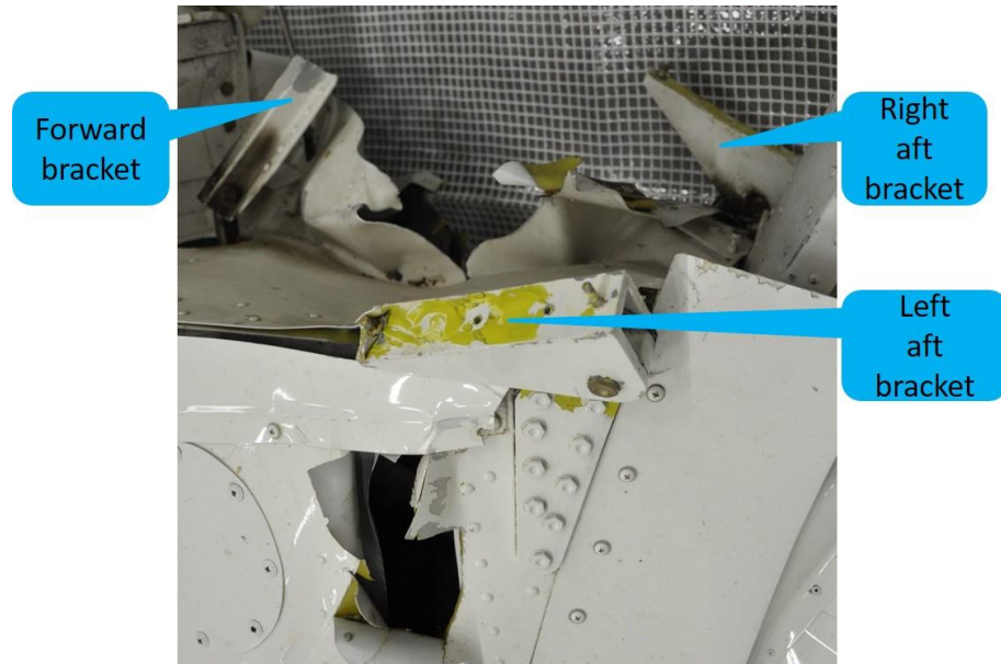
Figure 40. The stabiliser's attachments.
