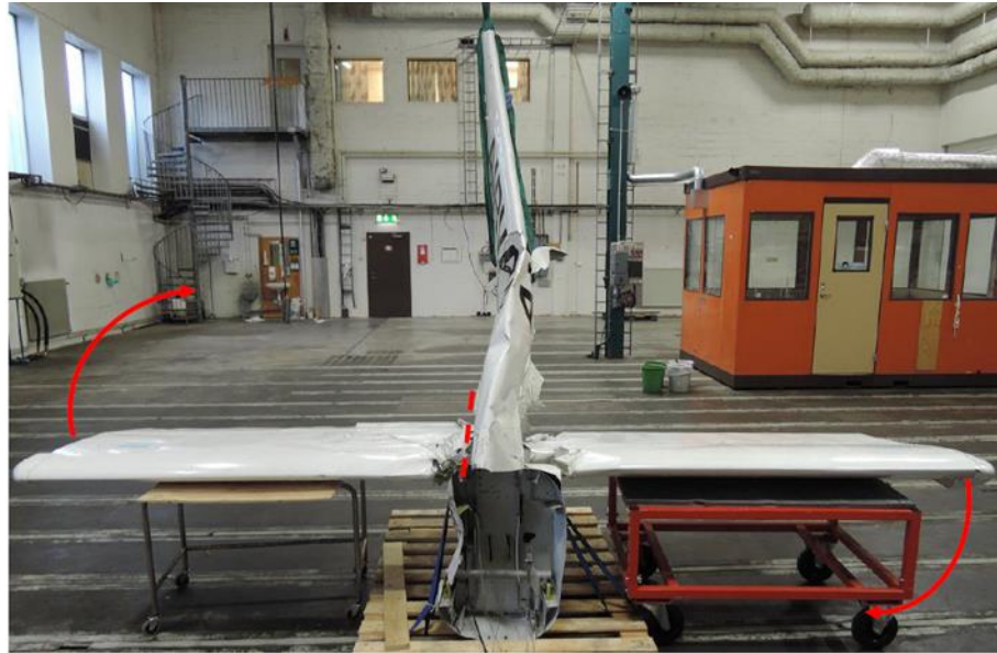
Figure 46. Sequence of failure of the stabiliser and the fin.
