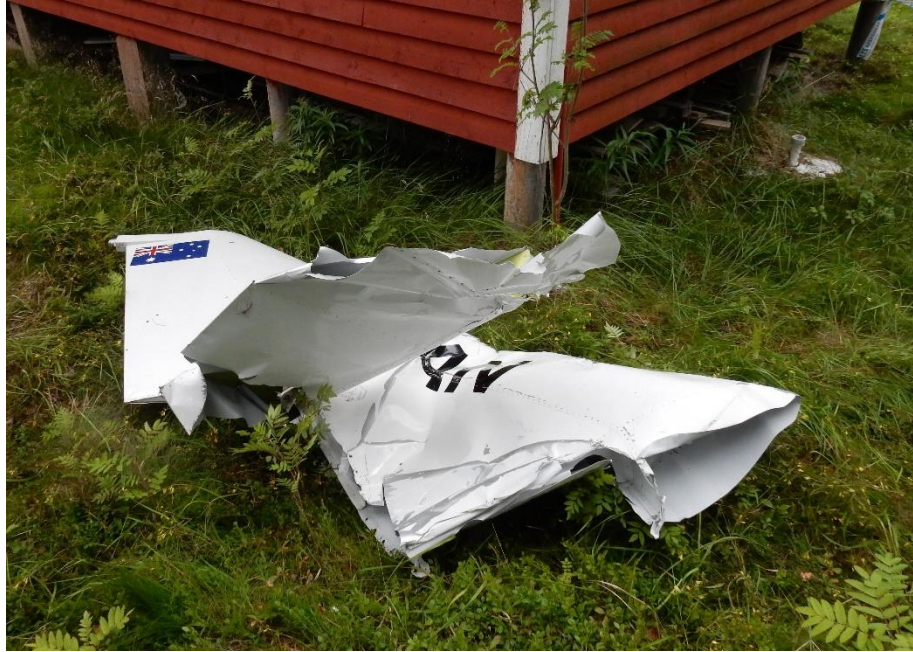
Figure 28. The broken off fin of the aeroplane.
