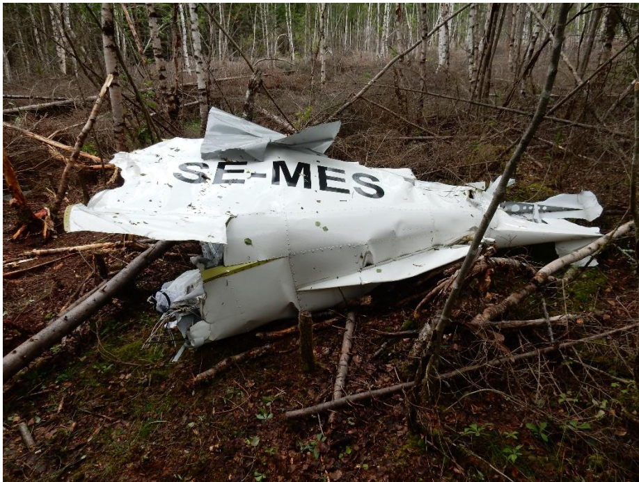
Figure 27. The tail section cut off by the fire and rescue service.
