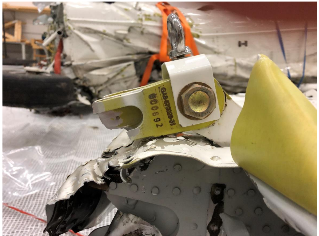
Figure 37. The broken attachment to the right wing strut.
