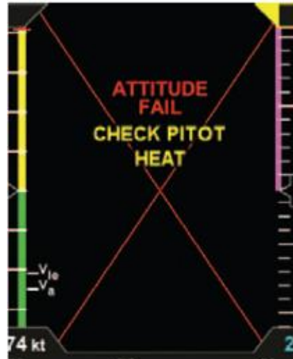
Figure 14. Indication on the primary flight information display in the event of a blocked pitot or static system. Image: Aspen Avionics Inc.
