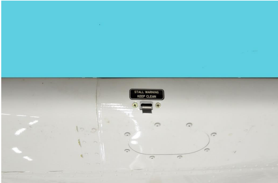
Figure 15. Stall warning vane on the wing.
