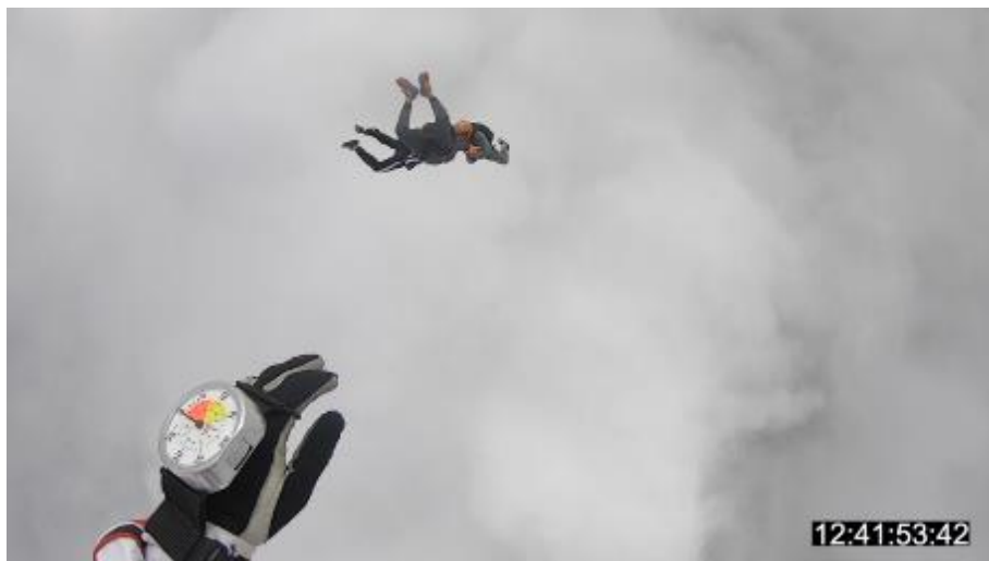
Figure 66. The parachutist with the camera leaves the aeroplane at approx. 12:41:53, the altimeter shows 4,000 m (needle at 0). The transponder altitude at 12:41:51 local time is 4,092 m. Picture: Umeå Parachute Club.
