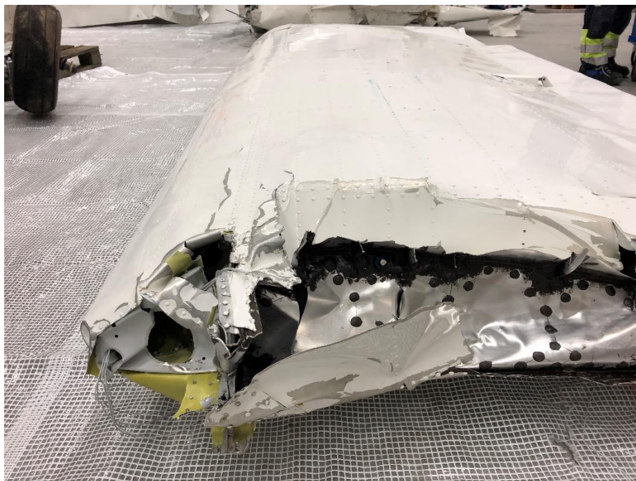
Figure 36. Upper surface of the outer section of the right wing.
