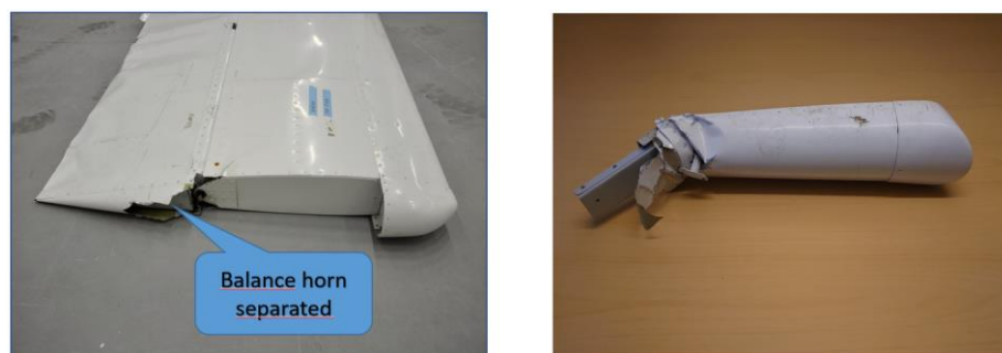
Figure 44. Left picture: Stabiliser and elevator with the balance horn separated. Right picture: The separated balance horn.
