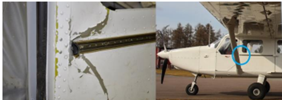
Figure 55. Left picture: Shows damage to the fuselage at the forward position of the door when it is open. Right picture: Marking by SHK that shows the position of the damage on the fuselage. Photo: Krister Karlsmoen.
