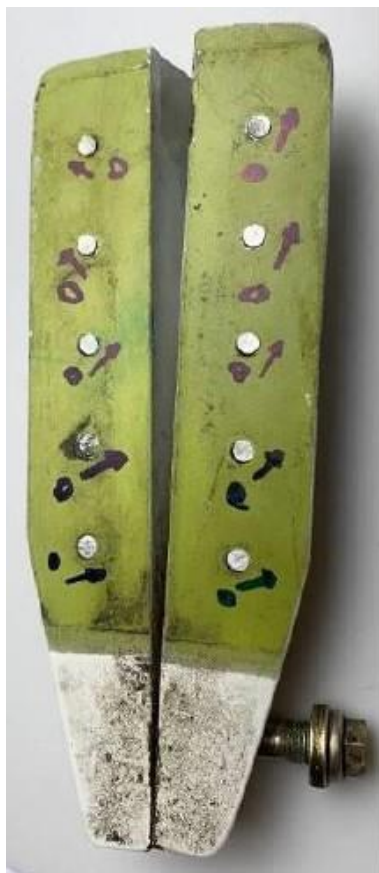
Figure 43. Bracket for front attachment of the stabiliser.
