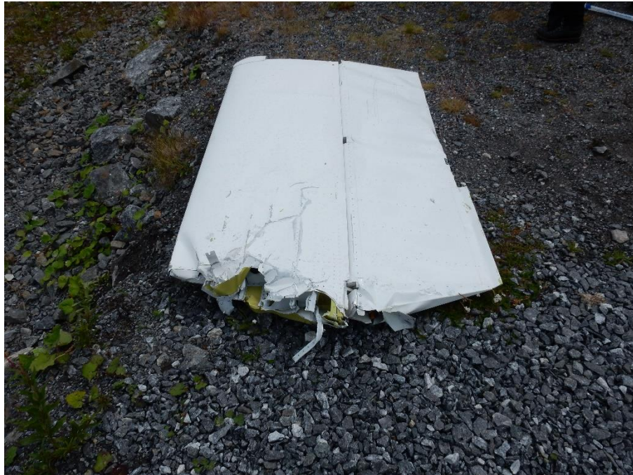
Figure 32. The right section of the stabiliser was salvaged from the Ume River.
