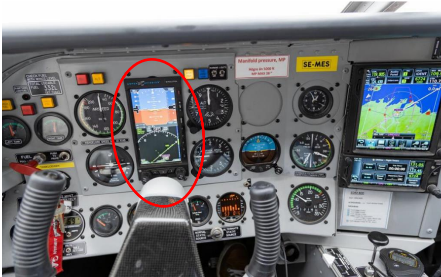
Figure 12. The flight instruments in SE-MES, with the Aspen PFD screen (marked with red ring by SHK) and the conventional flight instruments. Photo: Klas Sjöberg.
