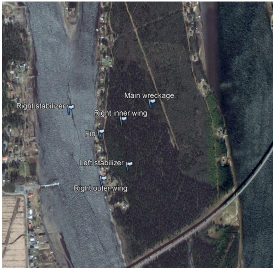
Figure 33. The accident site with the location of the parts of the wreckage. Photo: Google Earth: © Lantmäteriet Ref. no. R61749_190001.
